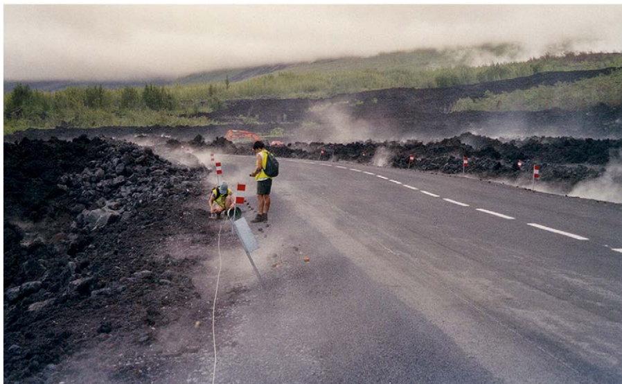
Fig. 2. Picture showing measurements on a two-month old lava flow. Self-potential data were measured along the national road. This one has just been rebuilt on top of the lava flow. The water vapour field on the lava flow is due to the heating of the meteoric water that percolates through the still hot lava flow.
