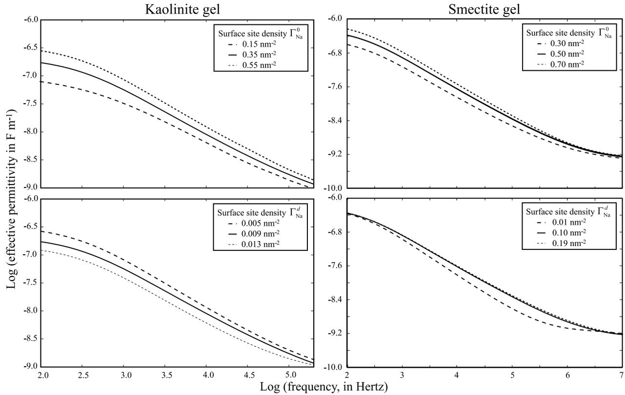
**Figure 8.** Sensitivity analysis for kaolinite and smectite for different values of the salinity, cation exchange capacity (CEC), and surface site densities in the Stern and diffuse layers (see other parameters in Table 4).
