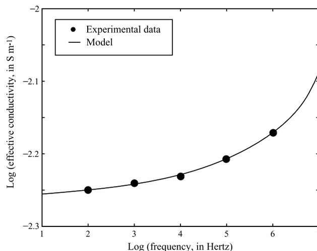
**Figure 18.** Comparison between the experimental data of *Scott et al.* [1967] and the prediction of the model based on the volume averaging approach concerning the effective conductivity (in S m<sup>-1</sup>) (see parameters in Table 9).
