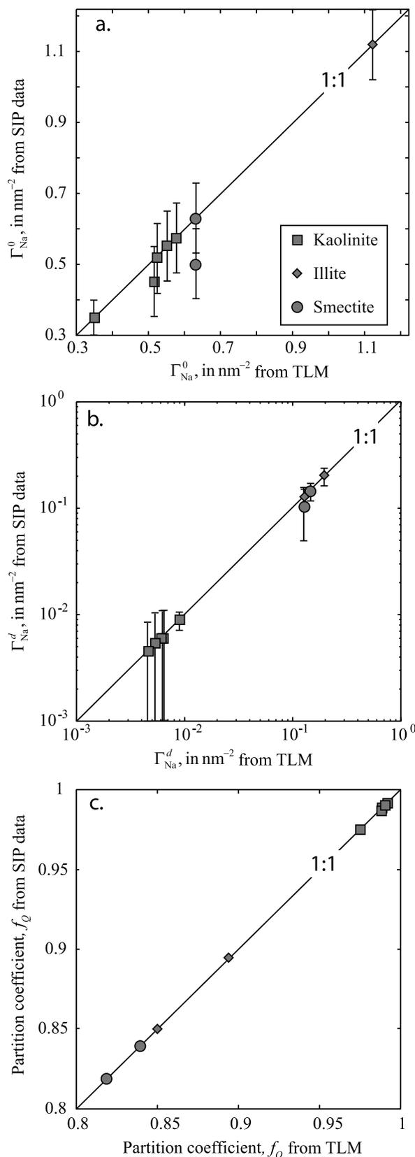
**Figure 19.** Comparison between the surface site densities (a) in the Stern layer and (b) in the diffuse layer determined from the spectral induced polarization data and those determined from the triple layer model. (c) Comparison for the partition coefficient.
