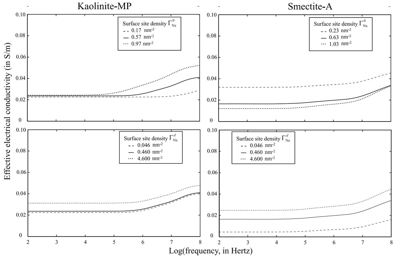
**Figure 10.** Sensitivity analysis for kaolinite and smectite for different values of the surface site densities in the Stern and diffuse layers (see other parameters in Table 8).
