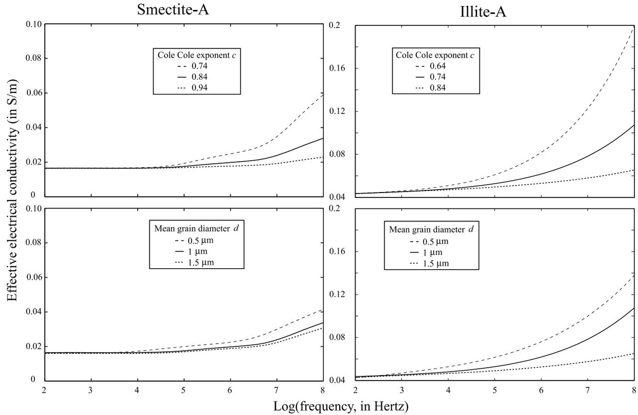
**Figure 9.** Sensitivity analysis for smectite and illite for different values of the Cole-Cole exponent and mean grain diameter assuming that the grain size distribution is given by a Cole-Cole distribution (see other parameters in Table 8).
