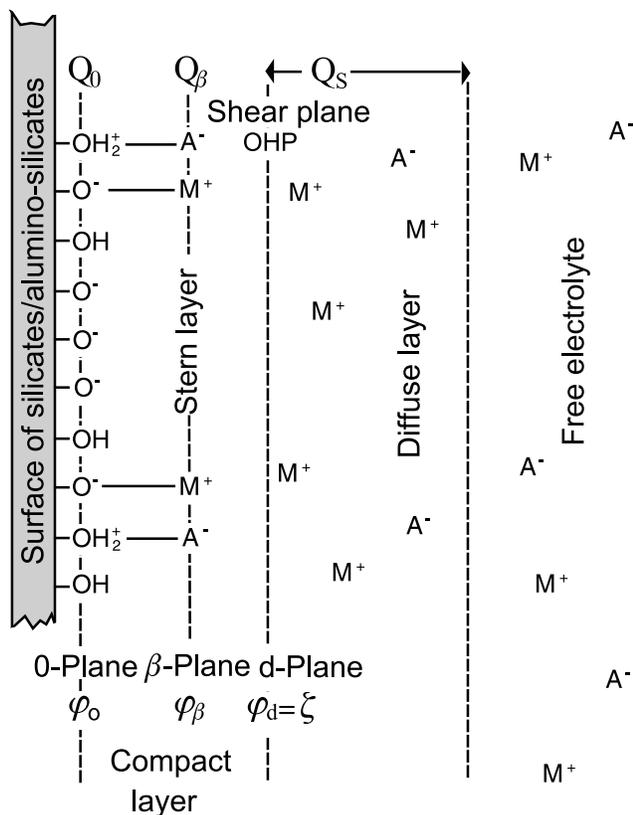
**Figure 2.** Sketch of the electrical triple-layer model, here for kaolinite (modified from *Leroy and Revil* [2004]). The symbol M represents the metal cations (e.g.,  $\text{Na}^+$  or  $\text{K}^+$ ) and A represents the anions (e.g.,  $\text{Cl}^-$ ). The OHP plane represents the Outer Helmholtz Plane, which coincides here with the shear plane along which the  $\zeta$  potential arising in electrokinetic phenomena is defined.
