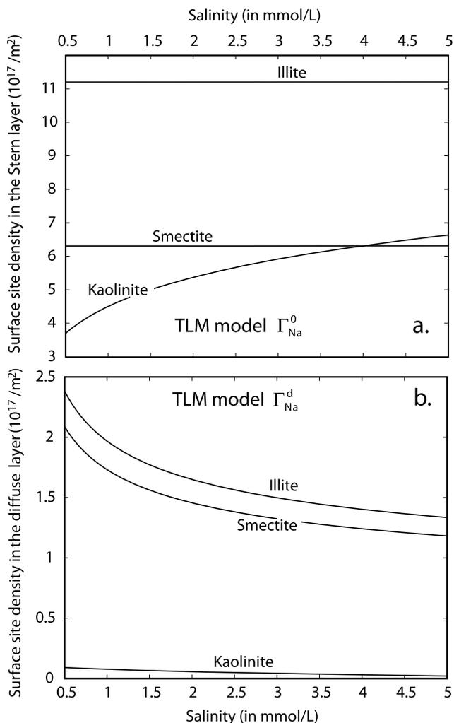
**Figure 3.** Computation of the surface site densities of counterions (a) in the Stern layer and (b) in the diffuse layer. We use the Triple Layer Model (TLM) described in section 2 (pH = 5.5, NaCl solution).
