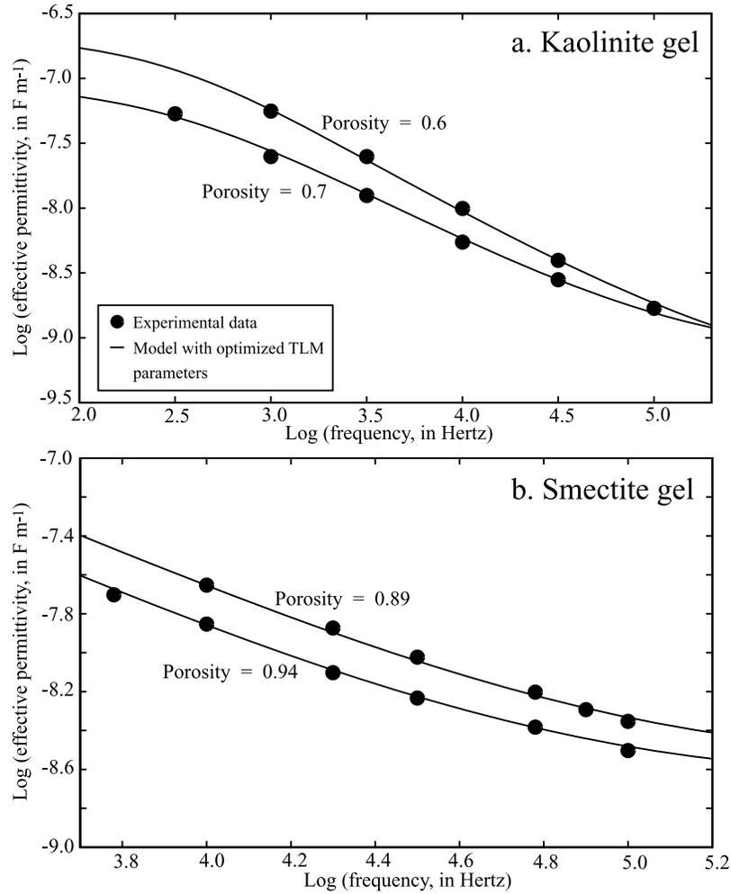
**Figure 12.** Comparison between the experimental data of *Lockhart* [1980a, 1980b] and the prediction of the differential effective medium approach for the effective permittivity (expressed in  $\text{F m}^{-1}$ ) using the TLM parameters of Table 4 at the salinity and pH ( $\sim 5.5$ ) of the pore water solution. (a) Kaolinite. (b) Smectite.
