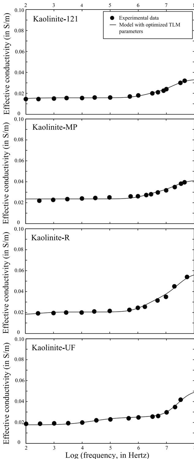
**Figure 14.** Comparison between the data of *Arulanandan* [1969] and the prediction of the differential effective medium approach for kaolinite concerning the effective conductivity (in  $\text{S m}^{-1}$ ) using the measured PSD.
