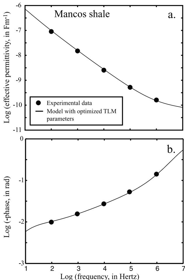
**Figure 17.** Comparison between the experimental data of *Scott et al.* [1967] and the prediction of the volume averaging approach (see parameters in Table 9). (a) Effective dielectric constant. (b) Phase angle (see equation (30)).
