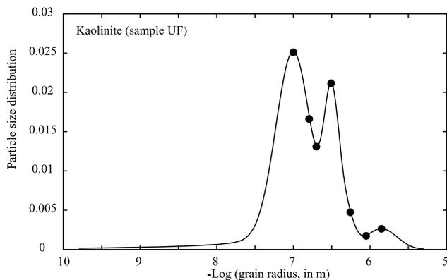
**Figure 13.** Example of particle size distribution (PSD) corresponding to the kaolinite core sample UF. Experimental data from *Arulanandan* [1969]. The PSD is fitted by the sum of two log normal distributions and a Cole-Cole distribution.
