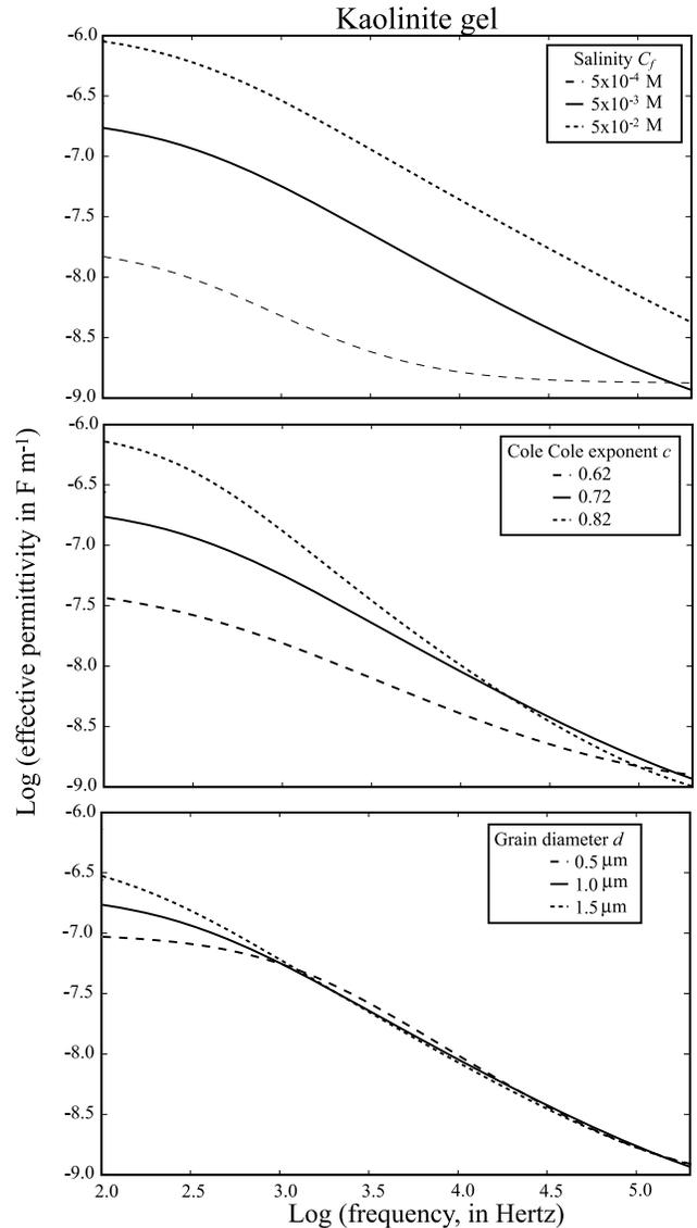
**Figure 7.** Sensitivity analysis for a kaolinite gel for different values of the Cole-Cole exponent and mean grain diameter assuming that the grain size distribution is given by a Cole-Cole distribution (see other parameters in Table 4).
