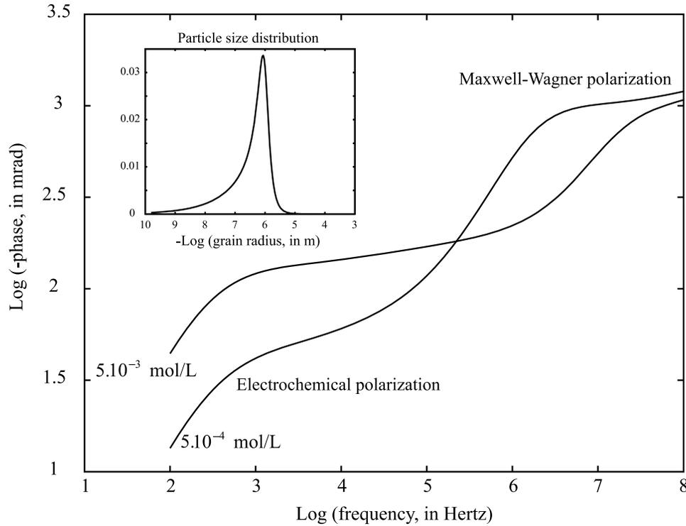
**Figure 6.** Prediction of the phase as a function of the frequency for kaolinite at two salinities (input parameters given in Table 3). We show also the domains dominated by the electrochemical polarization at low frequencies and the Maxwell-Wagner polarization at high frequencies.
