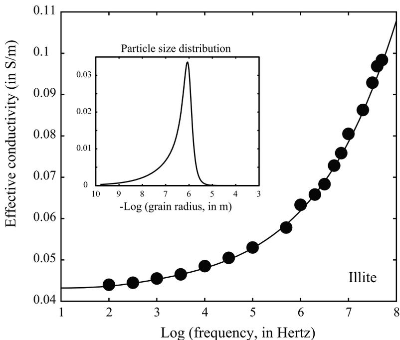
**Figure 15.** Comparison between the experimental data of *Arulanandan* [1969] and the prediction of the differential effective medium approach concerning the effective conductivity (in  $\text{S m}^{-1}$ ) for illite. The PSD being unknown, we use a Cole-Cole distribution for the PSD (see the insert and Table 8).
