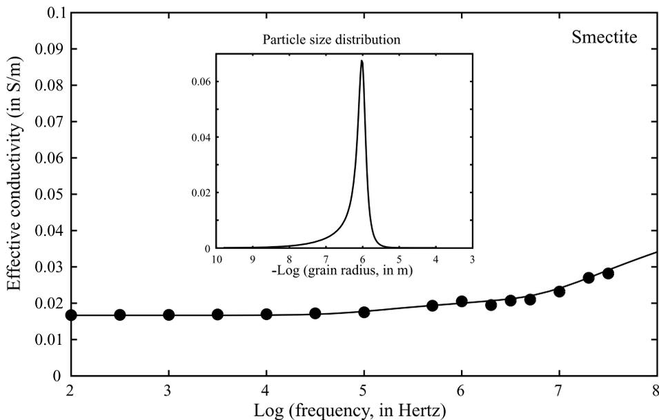
**Figure 16.** Comparison between the experimental data of *Arulanandan* [1969] and the prediction of the differential effective medium approach for a Na-montmorillonite (smectite). The PSD being unknown, we use a Cole-Cole distribution for the PSD (see the insert and Table 8).
