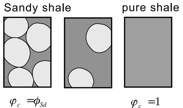
**Figure 11.** Sandy or silty shales are formed by silt and/or sand grains immersed into a clayey matrix with its own porosity. The volumetric clay content  $\phi_c$  is bounded by two values corresponding to two limiting cases. The first one is the case where a silt (or a sand) is completely infiltrated by clays with their own porosity. The second limiting case is the (usually fictitious) case of a pure shale without silt or sand grains immersed in the clay matrix.
