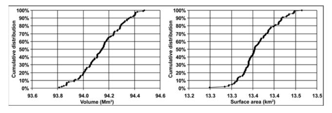
Fig. 11 Cumulative distribution of reservoir volume and area for a water elevation equal to 494.5 m (simulations outputs).
