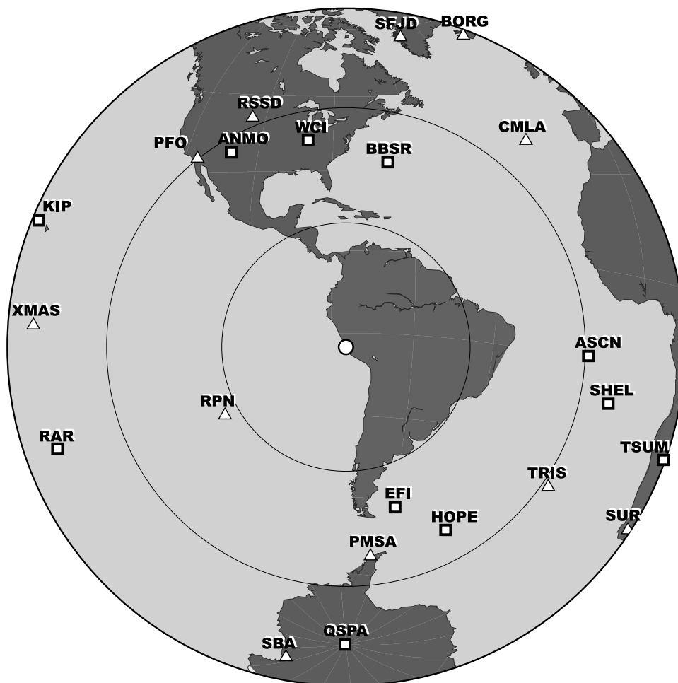
Figure 2. Squares and triangles give the position of the teleseismic stations for which P or P and SH waves have been processed and used for the inversion. Concentric circles are shown every 30^\circ of azimuthal distance from the epicenter.
