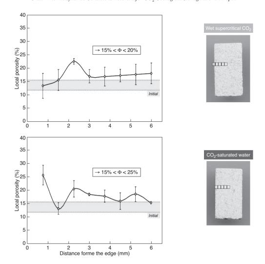
Figure 11 Cross-sections with localization of the areas chosen for SEM-BSE image analysis (left) and corresponding local porosity profiles (right) through the Lavoux limestone exposed to wet supercritical  $CO_2$  (above) and to  $CO_2$ -saturated water (below). The grey area with dashed lines corresponds to the initial local porosity range (14 $\pm$ 2%).
