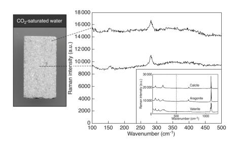
Figure 8 Raman spectra from the edge and the middle of the Lavoux limestone samples exposed to wet supercritical  $CO_2$  (above) and to  $CO_2$ -saturated water (below) during one month. The Raman spectra for the three calcium carbonate polymorphs are shown in the lowermost part. The Raman intensity is given in arbitrary units (a.u.).
