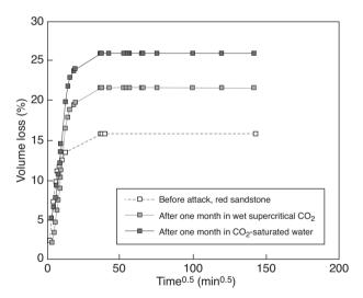
Figure 15 Evolution of the volume loss *versus*  $\sqrt{t}$  obtained with the water diffusion tests for the Adamswiller sandstone before exposure and after one month in wet supercritical  $CO_2$  and in  $CO_2$ -saturated water. The plateau corresponds to the porosity.
