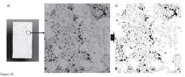
Sample cross-section a), grey-scale SEM-BSE images b) and binarized BSE image c) of the Lavoux limestone before  $CO_2$  exposure. The proportion of the black part of the image corresponds to the local two-dimension porosity. Based upon estimates with a series of few binarized BSE images, the local porosity of the sound limestone is  $14\pm2\%$ .
