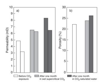
Evolution of the Lavoux limestone permeability deduced from water permeability measurements a) and porosity from Mercury Intrusion Porosimetry b) after exposure to wet supercritical CO<sub>2</sub> and CO<sub>2</sub>-saturated water during one month under reservoir conditions.
