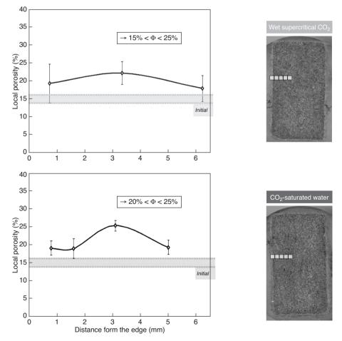
Cross-sections with localization of the areas chosen for SEM-BSE image analysis (left) and corresponding local porosity profiles (right) through the Adamswiller sandstone exposed to wet supercritical  $CO_2$  (above) and to  $CO_2$ -saturated water (below). The grey area with dashed lines corresponds to the initial local porosity range (15 $\pm$ 1%).
