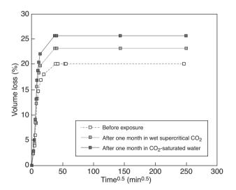
Figure 6 Evolution of the volume loss *versus*  $\sqrt{t}$  obtained with the water diffusion tests for the Lavoux limestone before exposure and after one month in wet supercritical CO<sub>2</sub> and in CO<sub>2</sub>-saturated water. The plateau corresponds to the porosity.
