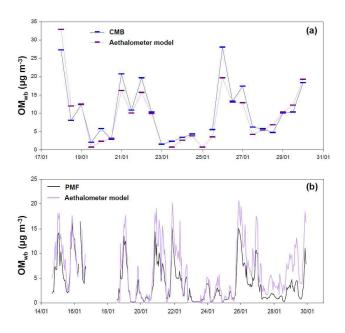
**Fig. 10.** Inter-comparisons of the time series of OM<sub>wb</sub> concentrations calculated by the different source apportionment models. (a) Outputs of the CMB and Aethalometer models (12h-averaged data, from 17 January 2009, 18:00 to 30 January 2009, 06:00). (b) Outputs of the AMS-PMF and Aethalometer models (15 minaveraged data, from 14 January 2009, 16:00 to 29 January 2009, 23:30).
