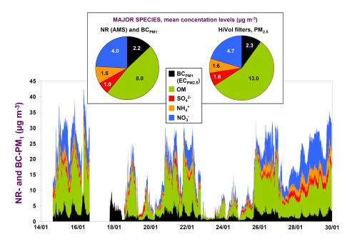
Fig. 1. Time series and mean concentration levels of the main components of the fine aerosol fraction during the period of study. Due to technical issues, AMS measurements are not available from 16/01 to 18/01. Mean PM<sub>2.5</sub> concentrations and BC<sub>PM1</sub> were calculated during the same periods than AMS measurements (upper panel).
