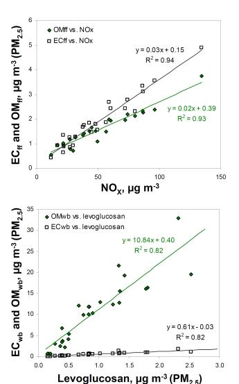
**Fig. 8.** Scatterplots of  $EC_{ff}$  and  $OM_{ff}$  as well as of  $EC_{wb}$  and  $OM_{wb}$ , as calculated by the Aethalometer model, versus  $NO_x$  and levoglucosan concentrations respectively.
