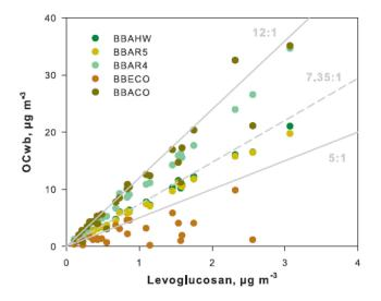
**Fig. 3.** Biomass burning organic carbon  $(OC_{wb})$  estimated using CMB modeling with the five selected biomass burning profiles as a function of levoglucosan. The dotted grey line represent the OC-to-Levoglucosan ratio recommended by Puxbaum et al. (2007) for European background environments, while grey lines as used here as indicators.
