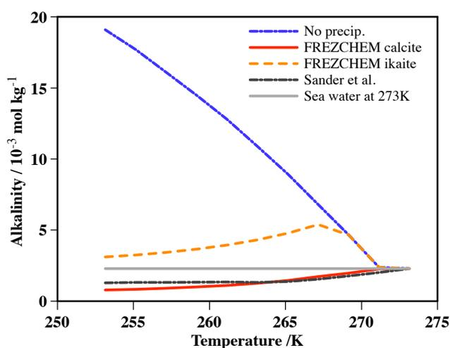
**Fig. 2.** Alkalinity  $A_T$  of the brine during the freezing of sea water. The definition is  $A_T = m(\text{OH}^-) + m(\text{HCO}_3^-) + 2m(\text{CO}_3^{2-}) + 2m(\text{CaCO}_3) + 2m(\text{MgCO}_3) - m(\text{H}^+)$ , where  $\text{CaCO}_3$  and  $\text{MgCO}_3$  represent dissolved ion pairs.
