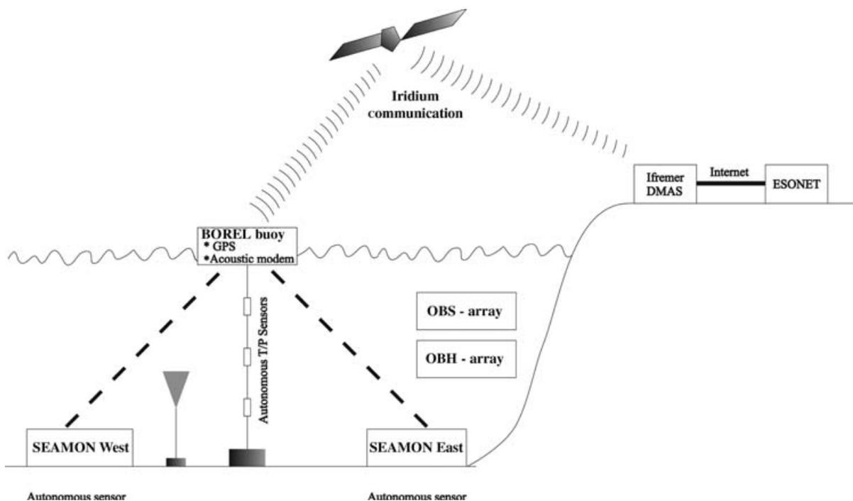
Figure 4: BOREL buoy that will assure data transmission relay between the SEAMON seabed stations and the Iridium satellite constellation
