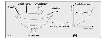
Fig. 2. Schematic representation of the hydrologic model. (a) Water balance model. (b) Area-depth relation.
