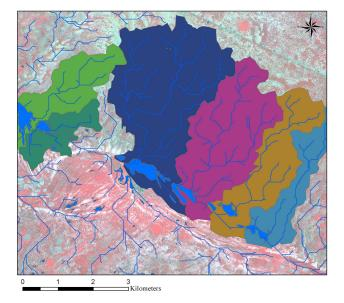
Fig. 4. Catchment area delineation using ASTER DEM. Ferlo valley, Senegal.
