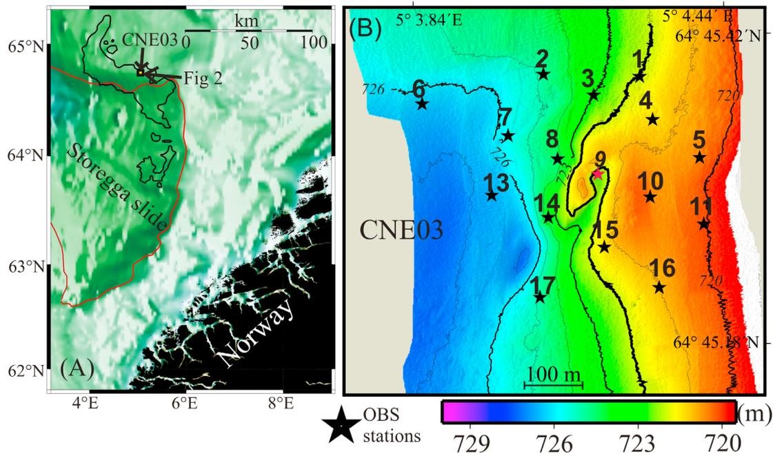
**Figure 1.** (a) Location and (b) bathymetry of the CNE03 pockmark at the mid-Norwegian continental margin. The CNE03 pockmark lies a few kilometers north from the Storegga slide (outlined in red in Figure 1a) and close to the northern limit of the prevalent BSR area (outlined in black in Figure 1a) [after Büinz *et al.*, 2003]. OBS sites are displayed around the pockmark. Only a limited amount of data from OBS 9 (at the center of the pockmark) was recovered.
