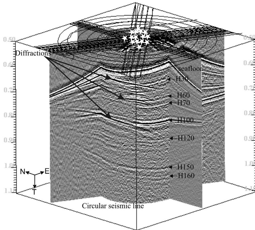
**Figure 3.** Selected seismic reflection sections from the OBS seismic experiment at the CNE03 pockmark showing the diffractions interfering with primary reflections. Arrivals from N–S, NW–SE, NE–SW, and circular seismic lines were recorded by an array of 15 OBSs (represented by stars). The seven seismic reflection events used for tomographic modeling are labeled.
