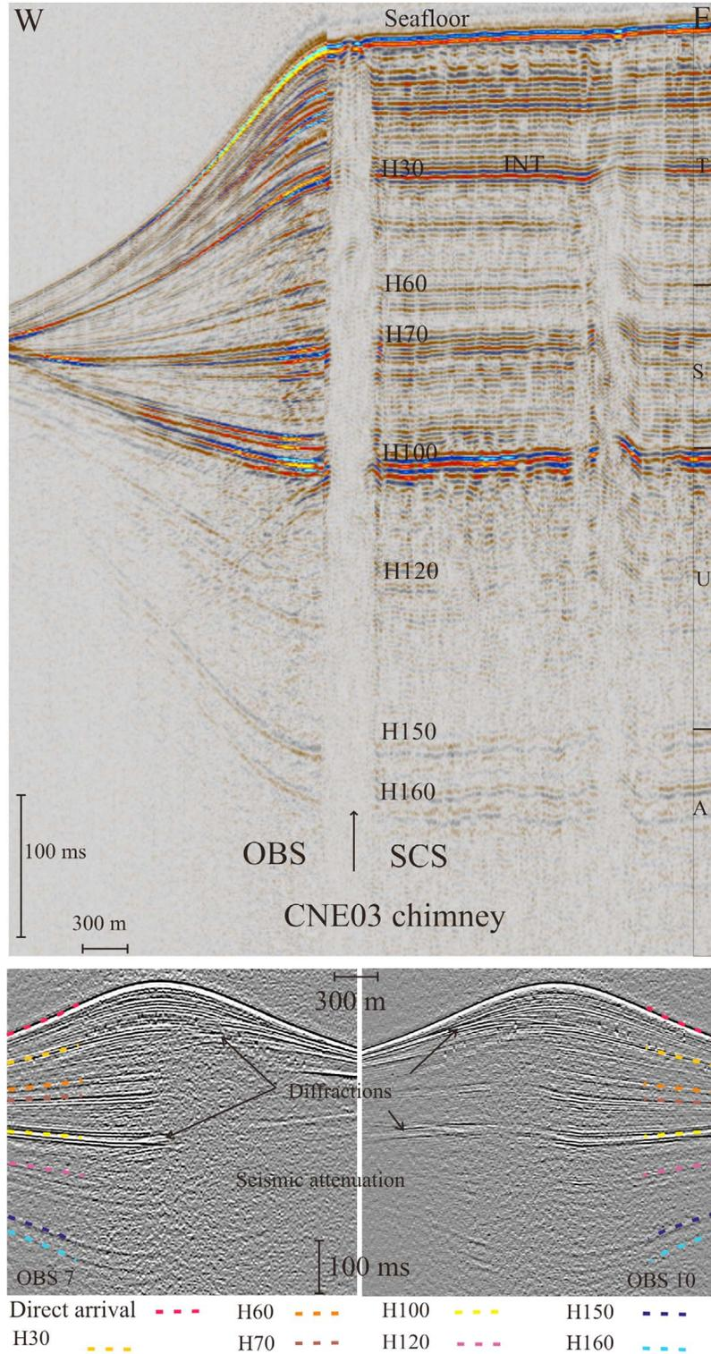
**Figure 4.** (top) Correlation between the OBS and streamer data. The interpreted reflectors have been correlated with the published seismic stratigraphy of the area [Rise *et al.*, 2006]. (bottom) OBSs 7 and 10 profiles recording from the western and eastern flanks of the chimney, respectively, show the seismic attenuation and diffractions impeding picking of the main reflectors at both sides of the chimney. The interpreted reflectors are indicated (dashed lines).
