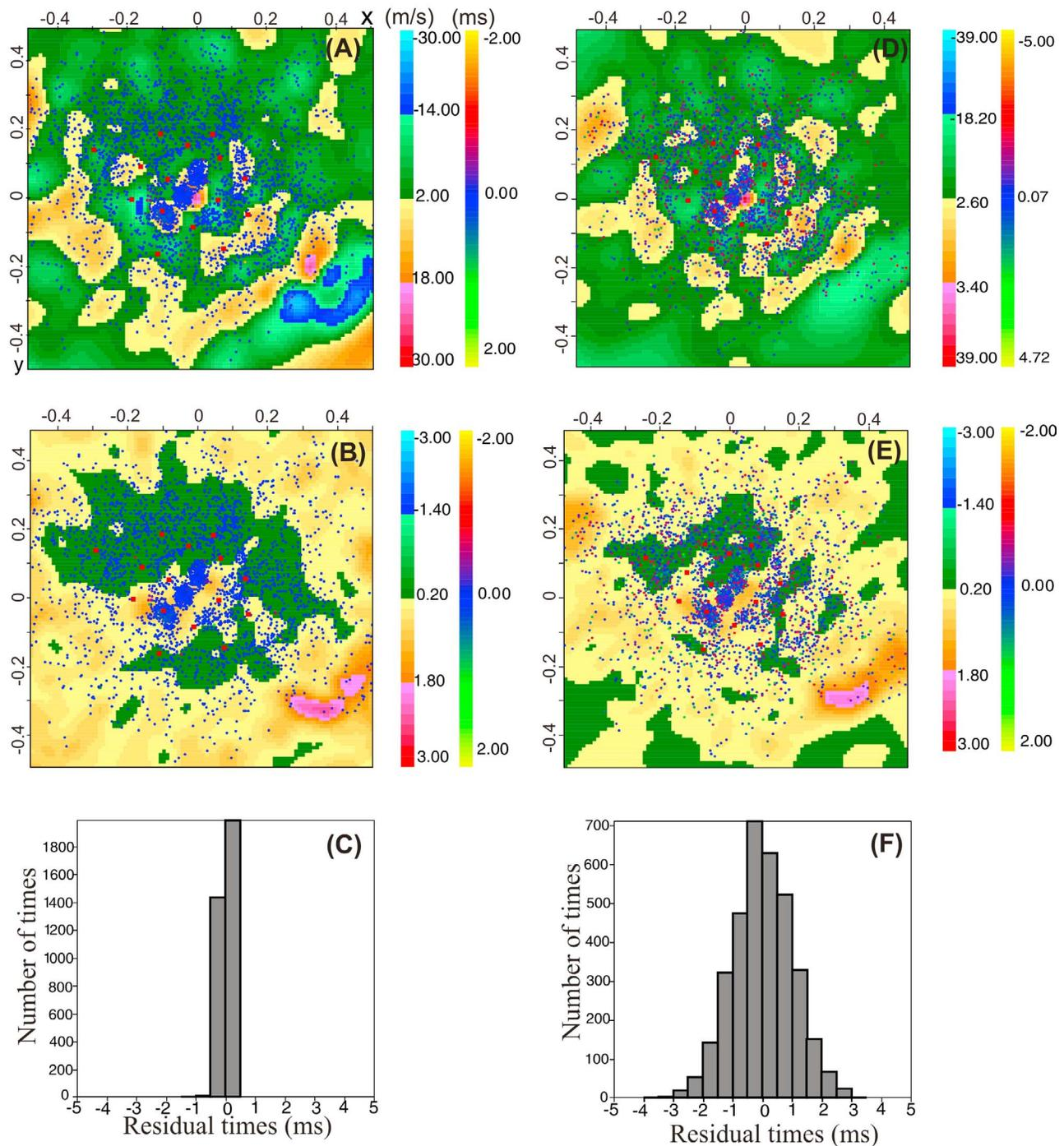
**Figure B6.** Uncertainty test 2: synthetic modeling completing the missing travel times for H70. (a and b) Top views show the velocity and interface depth differences after synthetic modeling. (d and e) The same random noise as for test 1 has been added to compare with the synthetics without noise. (c and f) Notice the changes in magnitude and distribution of the residuals after adding noise to the synthetic travel times by comparing histograms with and without noise.
