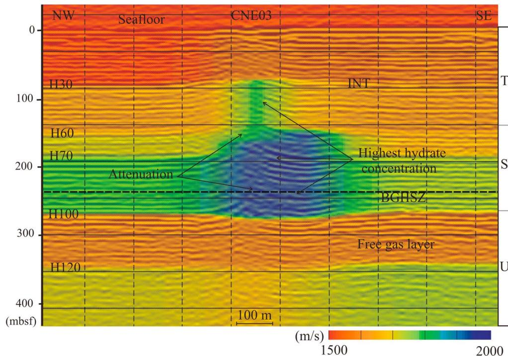
**Figure 9.** Inferred CNE03 chimney structure presented on a NW–SE oriented seismic reflection section (see Figure 2 for location) on which the  $V_p$  model has been overlain. The seismic attenuation is stronger at the western half of the chimney. The structural relief of reflectors increases only very slightly toward the base gas hydrate stability zone (BGHSZ).
