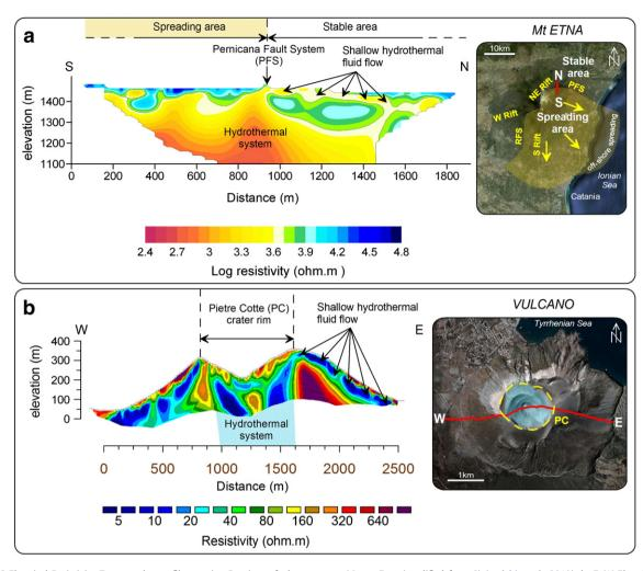
Fig. 5. a: N–S Electrical Resistivity Tomography profile crossing Pernicana fault system on Mount Etna (modified from Siniscalchi et al., 2010). b: E–W Electrical Resistivity Tomography profile crossing La Fossa cone of Vulcano (modified from Revil et al., 2008).
