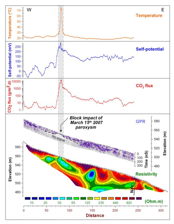
Fig. 2. Comparison between the temperature measurements (performed at a depth of 30 cm), the self-potential measurements, the soil CO<sub>2</sub> flux data, the ground penetrating radar data and the electrical resistivity tomography along the W–E profile shown in Fig. 1b. The temperature, the self-potential, and CO<sub>2</sub> anomalies coincide together with the area where the electrical conductive body reaches locally the ground surface at the block impact point.
