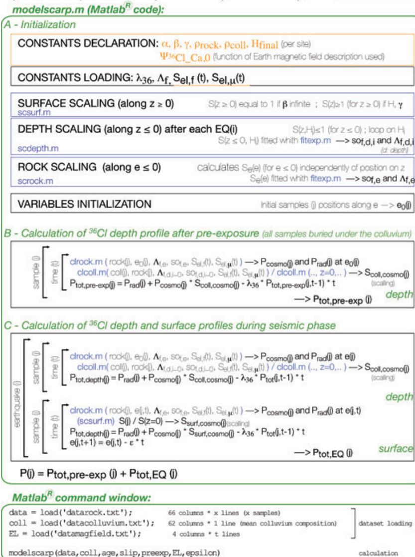
Figure B1. Schematic representation of the Matlab R modelscarp.m program given in Supplement 1. In orange, parameters that need to be modified for each site by the users. EQ stands for Earthquake; f for neutrons; \mu , for muons; j for the sample; i for the earthquake number; t for the time step; rock for the sample chemical composition; coll for the mean colluvial wedge composition; P_{cosmo} for the cosmogenic production; P_{rad} for the radiogenic production; epsilon for the erosion rate (in \text{mm yr}^{-1} ).
