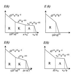
FIG. 1. Possible inertial regimes of energy spectral density in rotating MHD turbulence for Pm=1. The capital letters R, A, and K denote a rotating, Alfvén, or Kolmogorov turbulence.
