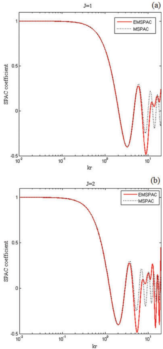
**Figure 1.** Comparing EMSPAC and MSPAC coefficients for  $M = 5$  for two different circles in the co-array,  $M$  is the number of stations and  $j$  is the number of the circle in the co-array. (a) Comparing the coefficients in the first circle,  $j = 1$ . (b) Comparing the coefficients in the second circle,  $j = 2$ .
