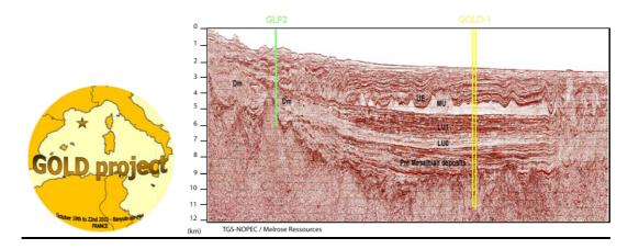
Position of the proposed GOLD drilling on seismic profile, at 2400 m water depth, 7.7 km of sédiments with 1 km of salt (transparent layer MU on profile) down to the crust record 30 Ma of high resolution earth history.
