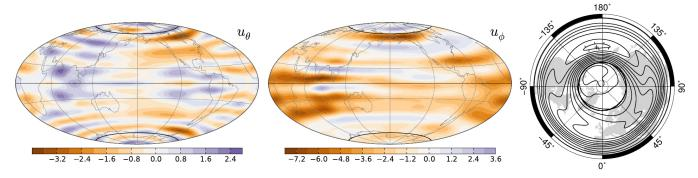
FIG. 3. Inverted flow  $\bar{\mathbf{u}}^{\pm}$  using  $\lambda_A = 8 \times 10^6$  averaged over the CHAOS-3 era. From left to right :  $u_{\theta}$  and  $u_{\phi}$  components in km/yr, and the stream-function  $\xi$  of the symmetric part  $\bar{\mathbf{u}}^+$  viewed from north-pole defined by  $\bar{\mathbf{u}}^+ = (\cos \theta)^{-2} \mathbf{r} \times \nabla \xi$ . The parallel coresponding to the trace of the TC is drawn (as well as  $\pm 20^{\circ}$ , related to table IV).
