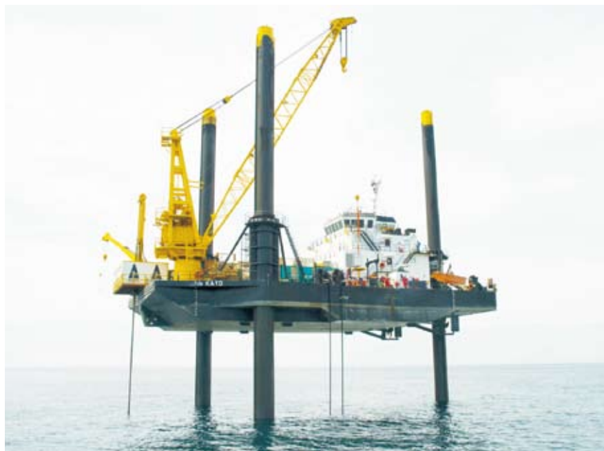
Figure 2. L/B Kayd (Montco Offshore, Inc.) outfitted with a commercial drill rig using coring tools developed and operated by DOSECC, Inc., during Expedition 313 while under direction from ESO. It stands in 35 m of water 45 km off the New Jersey coast.
