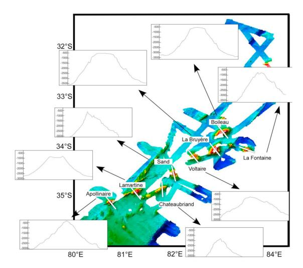
**Figure 4.** Morphologic profile of each seamount. White rectangles denote the location of cross sections on the chain of Dead Poets bathymetry. The vertical scale is similar for all the seamounts.
