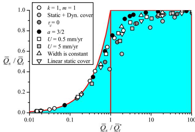
**Figure 11.** Effect of varying boundary conditions (discharge variability, uplift rate) and numerical model features (static and dynamic cover, variable width, linear static cover, incision exponent, critical shear stress) on the occurrence of hybrid channels in variable discharge simulations. If not specified in the legend, other parameters are  $m = 2, k = 1, U = 1$  mm/yr,  $a = 1$ , and exponential cover calculated as a function of sediment thickness.
