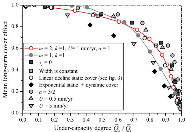
**Figure 13.** Long-term steady state cover effect as a function of the under capacity degree for various model parameters showing the consistent trend predicted whatever model features or boundary conditions. Note that linear decline static cover and exponential decline static cover predict almost the same results.
