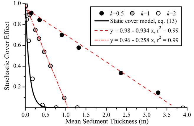
**Figure 15.** Relationships between stochastic cover effect and mean sediment thickness for different discharge variability. Each data point corresponds to the average values over 10,000 years obtained for a simulation with fixed bedrock channel geometry (i.e., slope can only vary because of alluvial deposits).
