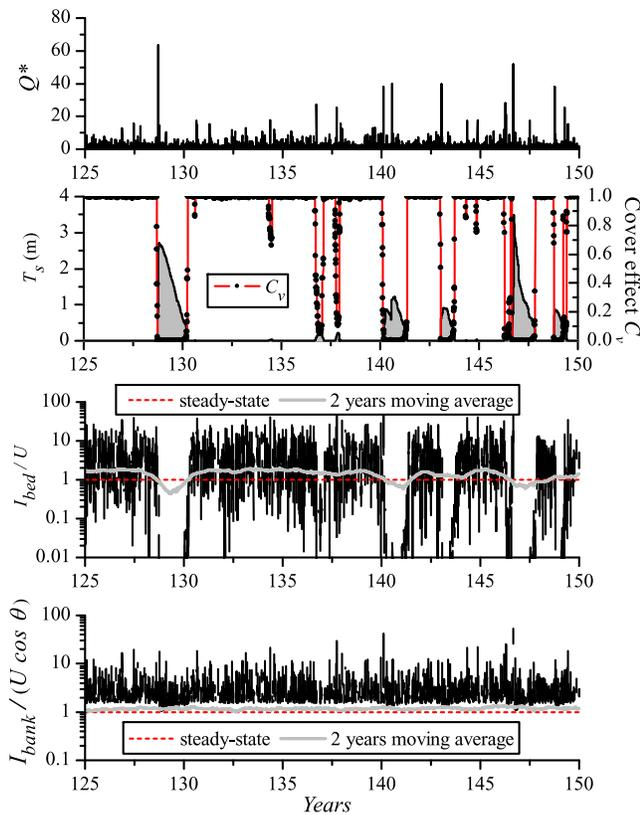
**Figure 7.** Temporal evolution of discharge, cover, and incision rates at daily time scales for  $m = 2$  at steady state. Large discharges deposit sediment that is progressively removed at time scales of months to years by lower discharges that are systematically net eroding (Figure 6). Note that the channel is rarely in partial cover effect configuration, but either on/off with respect to bed incision.
