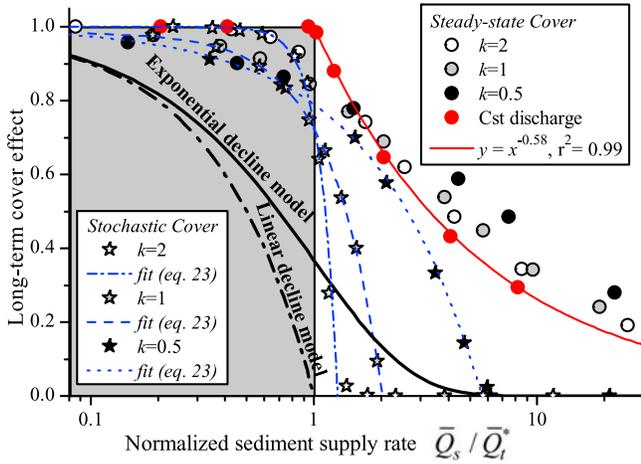
**Figure 14.** Steady state and stochastic cover effect as a function of the normalized sediment supply  $\bar{Q}_s/\bar{Q}_t^*$ . Using equation (23) to fit the stochastic cover data gives the following relationships: for  $k = 2$ ,  $y = 1 - 0.26 x^{5.5}$ ,  $r^2 = 0.99$ , for  $k = 1$ ,  $y = 1 - 0.26 x^{1.82}$ ,  $r^2 = 0.99$ , for  $k = 0.5$ ,  $y = 1 - 0.21 x^{0.90}$ ,  $r^2 = 0.99$ .
