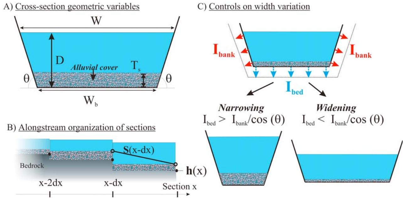
**Figure 2.** (a and b) SSTRIM numerical model geometry and variables and (c) width variations. Vertical dimensions are exaggerated. Bank angle is constant. Note that channel widening and narrowing affect water depth (for the same discharge) but also sediment thickness for the same volume per unit length of channel.
