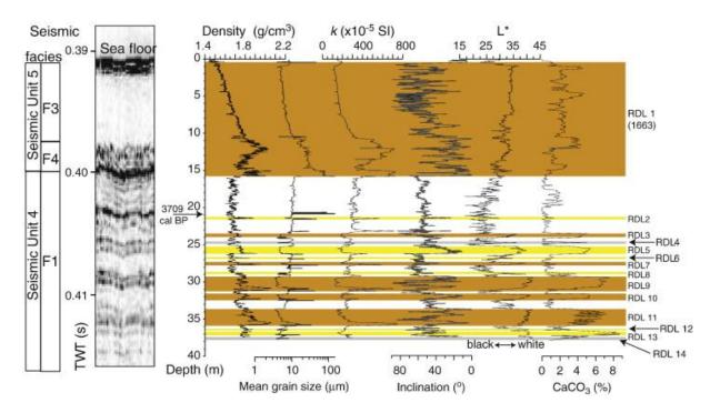
Fig. 9. Correlation of the seismic facies and Rapidly Deposited Layers (RDLs) identified at the sampling site of core MD99-2222 in the Saguenay Fjord. Two types of RDLs are distinguished (turbidites in yellow and turbidites capped by a hyperpycnite in orange) based on the physical properties (bulk density, diffuse spectral reflectance (L\*), grain size), carbonate content (CaCO<sub>3</sub>) and paleomagnetic data (low-field volumetric magnetic susceptibility (k) and inclination).
