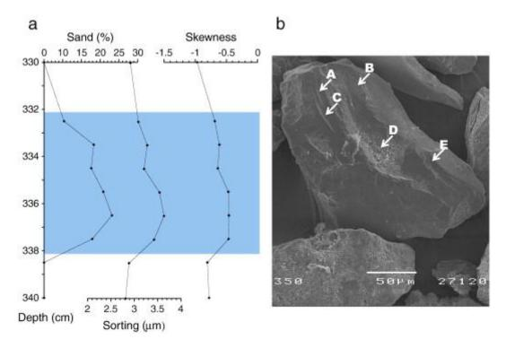
Fig. 13. Grain size signature of the sand layer overlying RDL 3 in the Reloncavi Fjord (a) and Scanning Electron Microscope (SEM) image of a typical quartz grain (b) from this layer characterized by dissolution features (A), fresh surfaces (B), percussion marks (C), adhering particle (D) and fresh surface (E).
