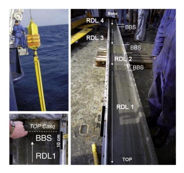
Fig. 12. Pictures of the Calypso CASQ corer on board the R/V *Marion Dufresne II* (left) and of core MD07-3108 Cq just after being opened on the deck (right). The Rapidly Deposited Layers (RDLs) are clearly contrasting with the Bioturbated Background Sediments (BBS). A detailed picture of the top of core MD07-3108 Cq before sampling reveals that RDL 1 is covered by less than 10 cm of BBS. A similar thickness of hemipelagic sediments was also observed in the companion surface core (see Fig. 15).
