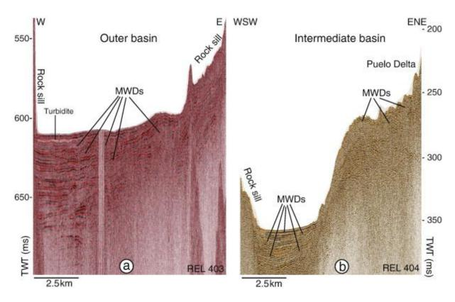
Fig. 6. Sparker (1 kHz) seismic profiles from the outer (a) and intermediate (b) basins of the Reloncavi Fjord illustrating the occurrence of mass wasting deposits (MWDs), rock sills and turbidites. The vertical scales are given in two-way-travel time (TWT).
