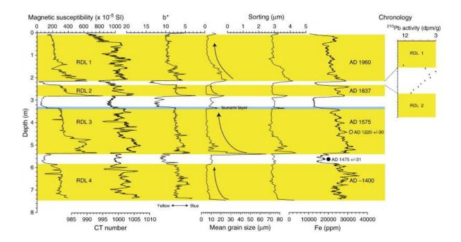
Fig. 11. RDLs in core MD07-3108 Cq. These layers were identified based on the physical properties (low-field volumetric magnetic susceptibility (k), CT number (primarily reflecting bulk density), diffuse spectral reflectance (b\*), grain size) and geochemistry (Fe content). Two types of RDLs are distinguished (four turbidites in yellow and a tsunami layer in blue). Ages obtained on a shell (black circle) and a wood fragment (white circle) are also illustrated.
