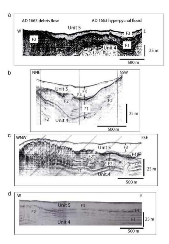
Fig. 4. Selection of four seismic reflection profiles from the inner basin of the Saguenay Fjord (see Fig. 2 for location) (4a, modified from Perret et al., 1995), in the distal part of the inner basin (4b and 4c, modified from Syvitski and Schafer, 1996) and in the middle of the inner basin (4d). Seismic units 4 and 5 of Syvitski and Praeg (1989) and Syvitski and Schafer (1996) are illustrated together with seismic facies F1, F2, F3 and F4 discussed in the text (this study).
