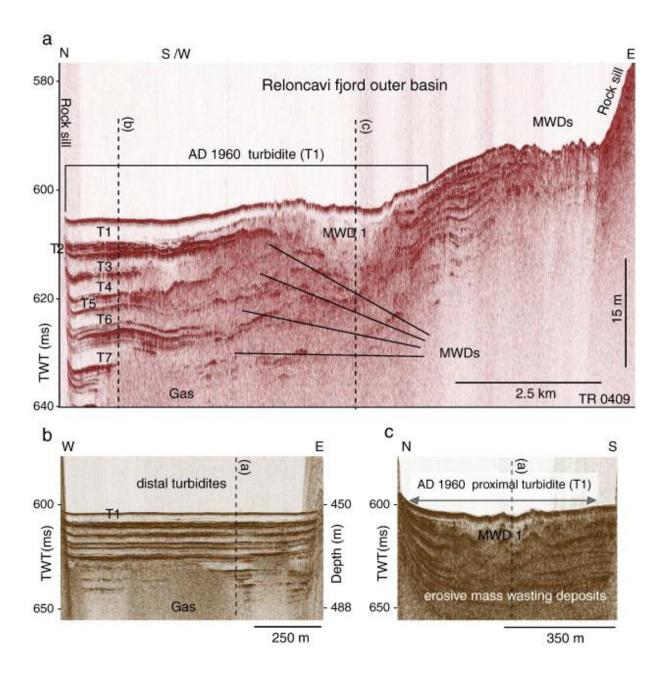
Fig. 7. Selection of pinger (3.5 kHz) seismic profiles from the outer basin of the Reloncavi Fjord illustrating the accumulation of mass wasting deposits (MWDs), seven large turbidites (T1 to T7) and the occurrence of free gas in the sediments. The vertical scale is given in two-way-travel time (TWT) and in meters (assuming a velocity of 1500 m s<sup>-1</sup>). Profiles a, b and c intersections are also shown.
