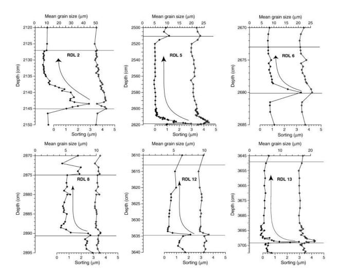
Fig. 10. Detailed grain size signature of RDLs (classical turbidites) from the Saguenay Fjord showing a fining-upward trend for each RDL.
