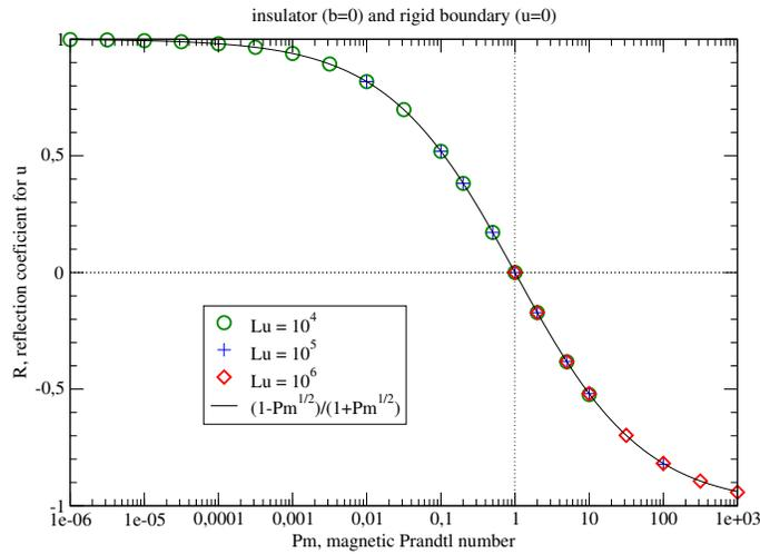
FIG. 1. Reflection coefficient for a one-dimensional Alfvén wave packet hitting an insulating boundary with normal incidence, as a function of  $Pm$  and for different magnetic Lundquist numbers  $Lu = V_a L / \eta$ . The theoretical value for plane waves  $R(Pm) = (1 - \sqrt{Pm}) / (1 + \sqrt{Pm})$  fits the data perfectly.
