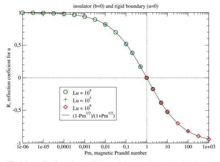
FIG. 1. Reflection coefficient for a one-dimensional Alfvén wave packet hitting an insulating boundary with normal incidence, as a function of Pm and for different magnetic Lundquist numbers  $Lu = V_a L/\eta$ . The theoretical value for plane waves  $R(Pm) = (1 - \sqrt{Pm})/(1 + \sqrt{Pm})$  fits the numerical simulation results perfectly.
