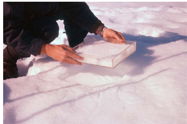
Figure 4. A pan filled with crushed ice was used to take sublimation/evaporation measurements. The pan is about 700 cm 2 in area and about 5 cm deep, made of Plexiglas. The pans were placed so that the top of the rim was flush with the snow or ice surface, and weighed before and after a 12 h exposure.
