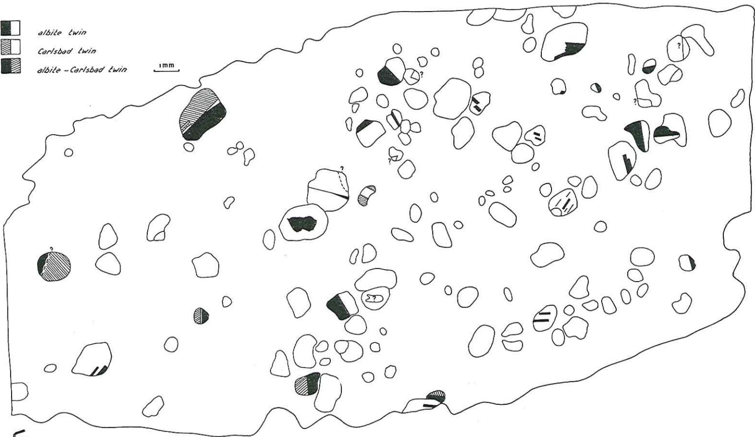
Fig. 15. Diagram of a thin section, indicating mode of occurrence and twinning of the albite porphyroblasts. St. Hugon schists (Sample T 257).
