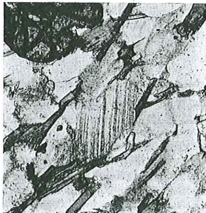
Fig. 21. Twinned plagioclase crystal, in which one set of lamellae is more altered than the other. Same sample as Fig. 20, plane-polarized light, 85 \times .
