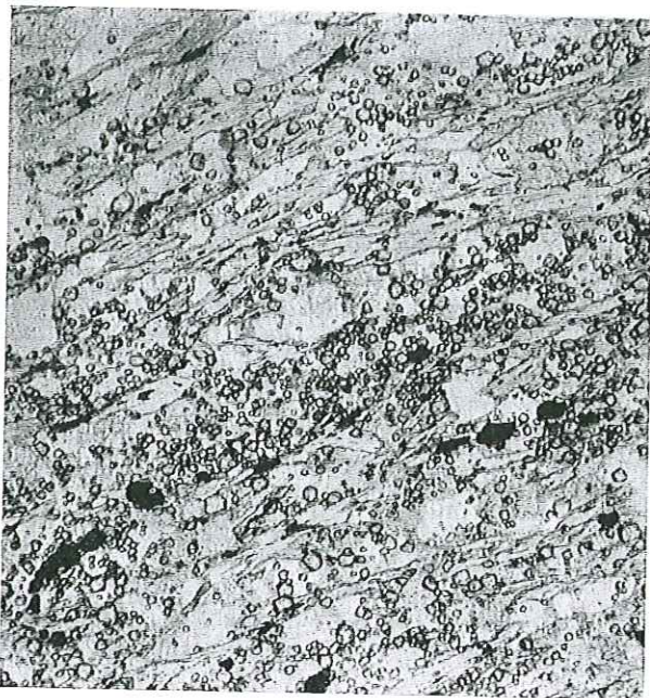
Fig. 28. Numerous very small garnets in garnet-biotite-schist of the Lac Crop formation. Sample 74559, plane-polarized light, 55 \times .
