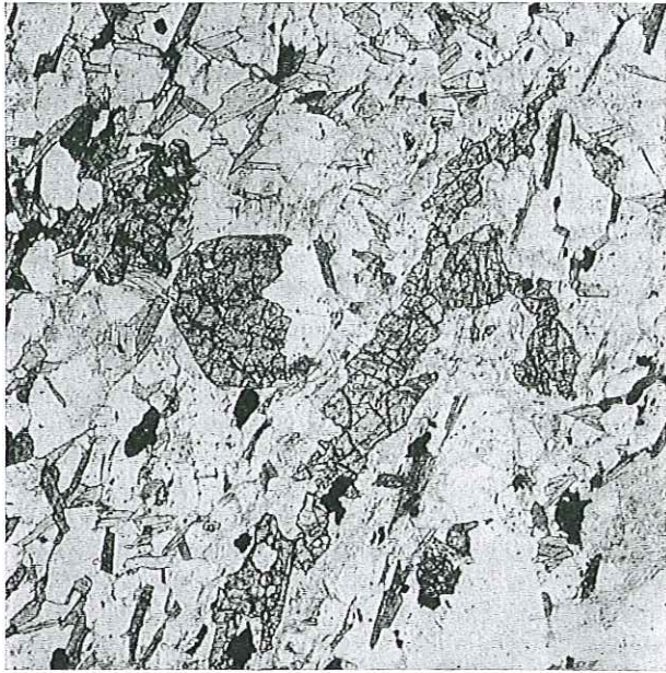
Fig. 30. Garnet (left) and staurolite (right) in biotite-schist of the Lac Crop formation. Same sample as Fig. 29, plane-polarized light, 30 \times .
