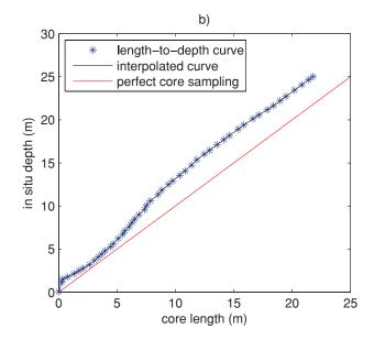
**Figure 3.** (a). *P*-wave velocity profiles: PENFELD *in situ* measurements (red), laboratory core measurements (dashed) + length-to-depth law correction (black) + environmental corrections (bold). (b) Length-to-depth relationship provided by the coring monitoring.
