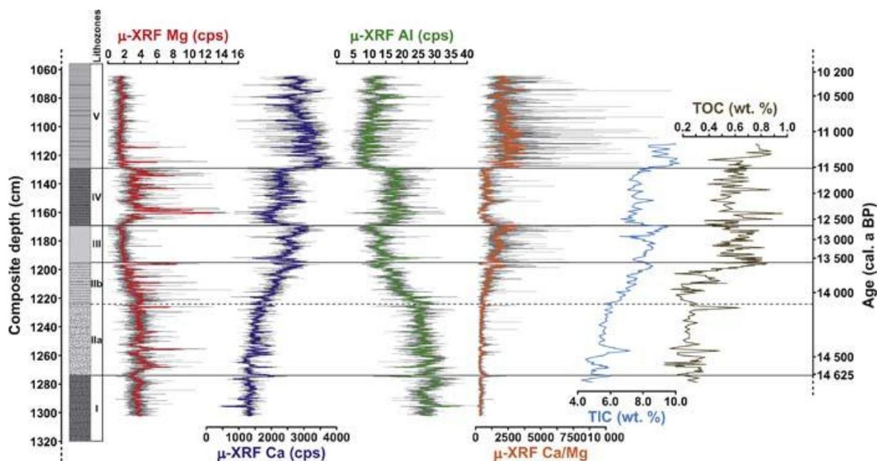
Figure 4. Results of  $\mu$ -XRF element scanning (thin lines: measurements at 200  $\mu$ m resolution; thick lines: 25-point running mean) and carbon geochemistry analyses obtained from the Lake Mondsee sediments across the Last Glacial–Holocene transition.  $\mu$ -XRF Mg counts reflect input of detrital dolomite and Al counts those of detrital siliciclastics, whereas Ca counts and TIC contents reflect variations in the abundance of endogenic calcite.
