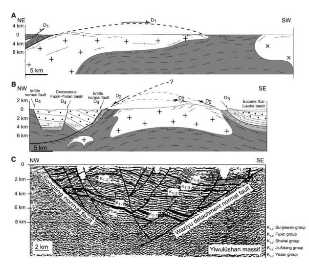
Fig. 3. Cross-sections though the Yiwulüshan massif and Fuxin–Yixian basin (the pluton roots are hypothetic. Location in Fig. 2 and figure captions are the same as in Fig. 2). A: Cross-section drawn parallel to the direction of the  $D_1$  southwestward deformation; B: Cross-section drawn parallel to the direction of the  $D_2$  northwestward deformation; C: Seismic profile parallel to the  $D_2$  extensional direction (re-interpretation from Wang et al., 1998b).
