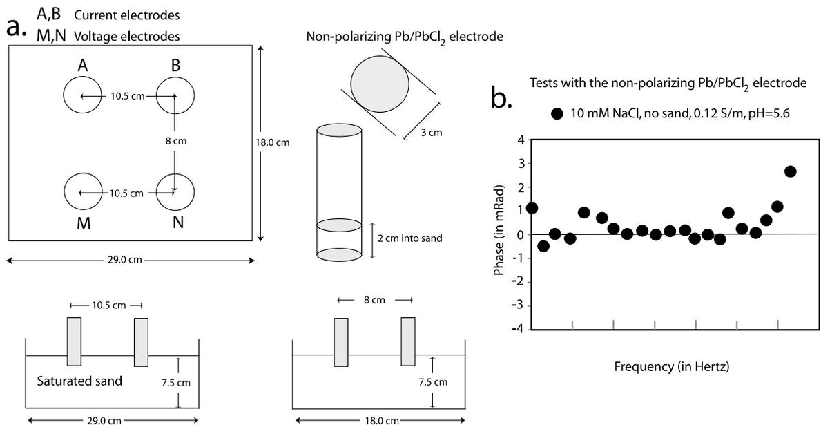
**Figure 5.** Experimental setting used to measure the complex resistivity. (a) The electrodes are non-polarizing Pb/PbCl<sub>2</sub> electrodes. They are used as current electrodes (A and B) and potential electrodes (M and N). The tank is made of plastic. (b) Test of the phase accuracy in absence of sand in a NaCl electrolyte.
