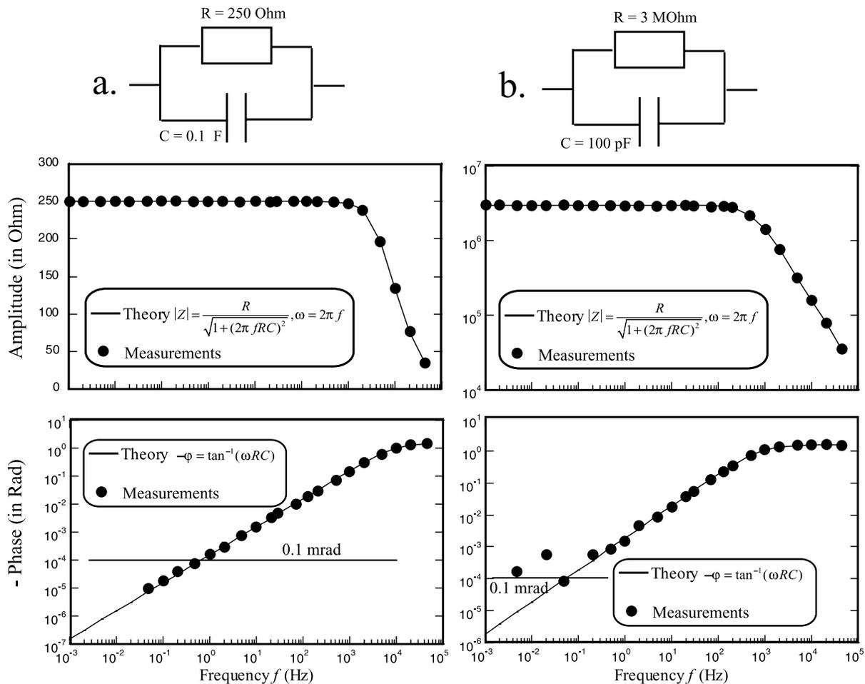
**Figure 4.** Test of the sensitivity of the impedance meter used in our experiments. We test the impedance meter by measuring the impedance of a known resistance in parallel to a known capacitance. (a) Test with a low resistance of  $250\text{ ohm}$  and a high capacitance  $0.1\text{ F}$ . (b) Test with a high resistance of  $3\text{ MOhm}$  and a small capacitance of  $100\text{ pF}$ .
