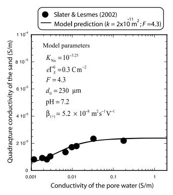
**Figure 11.** Tests of the Stern layer model. The input parameters for the predicted quadrature conductivity are the measured formation factor and the value of the specific surface conductivity of the Stern layer (at  $25\,^{\circ}$ C).
