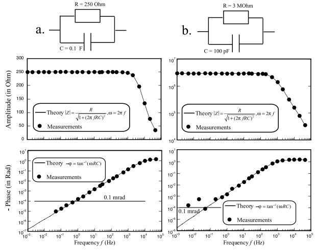
**Figure 4.** Test of the sensitivity of the impedance meter used in our experiments. We test the impedance meter by measuring the impedance of a known resistance in parallel to a known capacitance. (a) Test with a low resistance of 250 ohm and a high capacitance 0.1 F. (b) Test with a high resistance of 3 Mohm and a small capacitance of 100 pF.
