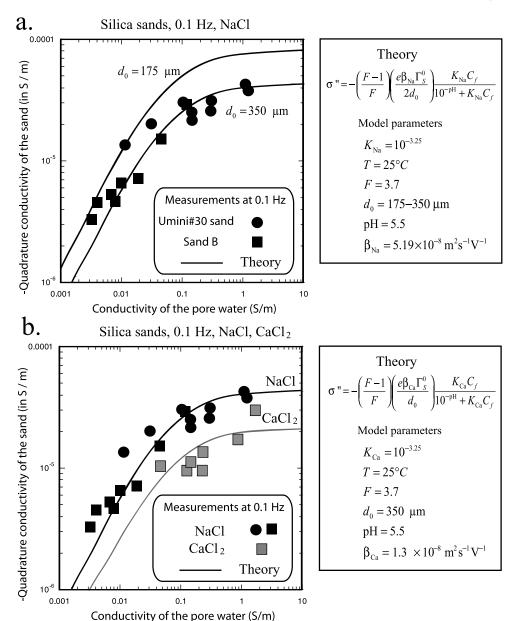
**Figure 8.** Comparison between the experimental data for the quadrature conductivity and the prediction of the model. Note that all the parameters entering into the model are fixed through independent estimates (listed on the lower left corner). The total site density is 5 sites per nm<sup>2</sup>. (a) For a sodium chloride solution. (b) Comparison with a CaCl<sub>2</sub> solution.
