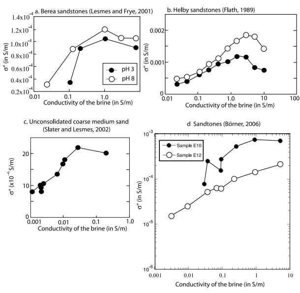
Figure 3. Salinity dependence of the quadrature conductivity. (a) Berea sandstone (Lesmes & Frye 2001). (b) Helby sandstones (Flath 1989). (c) Unconsolidated coarse medium sand (Slater & Lesmes 2002, sample G1, 1 Hz, 200 μm from permeability and formation factor estimates of table 1). (d) Börner (1992, 2006), sandstones (see Table 1). The lines are guides for the eyes. Note that for some samples, the decrease of the quadrature conductivity at high salinities may be due to membrane polarization.
