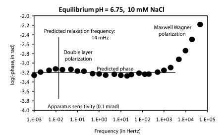
**Figure 6.** Example of phase data recorded over the full spectrum of frequencies (1 MHz to 40 kHz). The data exhibit clearly two polarization relaxations. The relaxation observed at low frequencies has been recently associated to the polarization of the Stern layer whereas the one at high frequencies is associated with the Maxwell–Wagner polarization.
