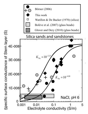
**Figure 9.** Specific surface conductivity of the Stern layer: comparison between the analytical model discussed in the main text and the experimental data (normalized quadrature conductivities and direct estimates). The model (25 °C, NaCl, plain line) is shown for two values of the sorption coefficient of sodium in the Stern layer.
