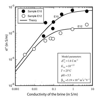
**Figure 10.** Test of the SLP model. The input parameters for the predicted quadrature conductivity are the measured permeability, the measured formation factor and the value of the specific surface conductivity of the Stern layer (at  $25~^{\circ}\text{C}$ ) computed from the analytical model.
