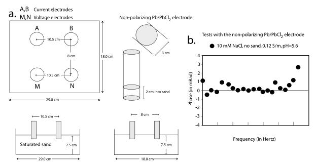
Figure 5. Experimental setting used to measure the complex resistivity. (a) The electrodes are non-polarizing Pb/PbCl<sub>2</sub> electrodes. They are used as current electrodes (A and B) and potential electrodes (M and N). The tank is made of plastic. (b) Test of the phase accuracy in absence of sand in an NaCl electrolyte.
