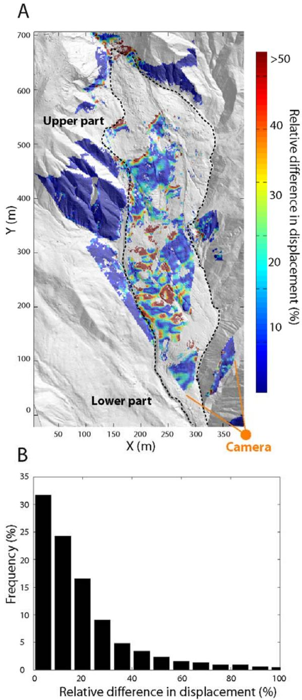
Fig. 17. Effect of the DEM on the ortho-rectification of the displacement field. (A) relative difference between the displacement field of the 1<sup>st</sup> June orthorectified with a DEM of 2007 and a DEM of 2009. (B) Histogram of the relative differences.
