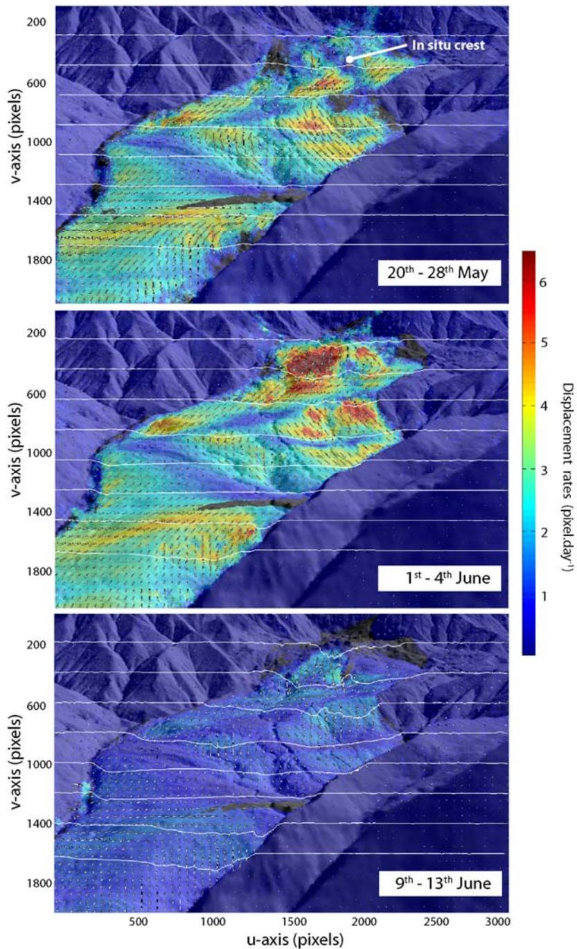
Fig. 8. Displacement rates amplitude (color) and displacement direction (arrows) in the image plane and cumulated displacements along 8 profiles crossing the landslide over the period the 20<sup>th</sup> May to the 25<sup>th</sup> June 2008. In order to highlight the displacement direction, the arrow length is normalized in each image.
