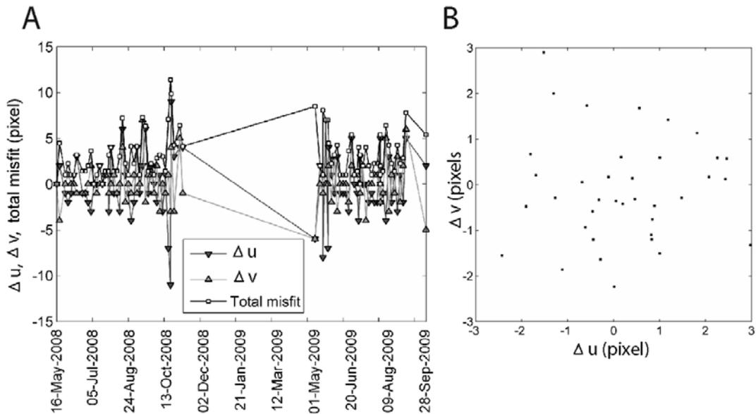
Fig. 16. Assessment of the accuracy of the camera orientation (A) Average homogenous components due to slight movement of the camera. (B) Residual  $\Delta u$  and  $\Delta v$  misfits between projected and observed GCPs after the least square minimization.
