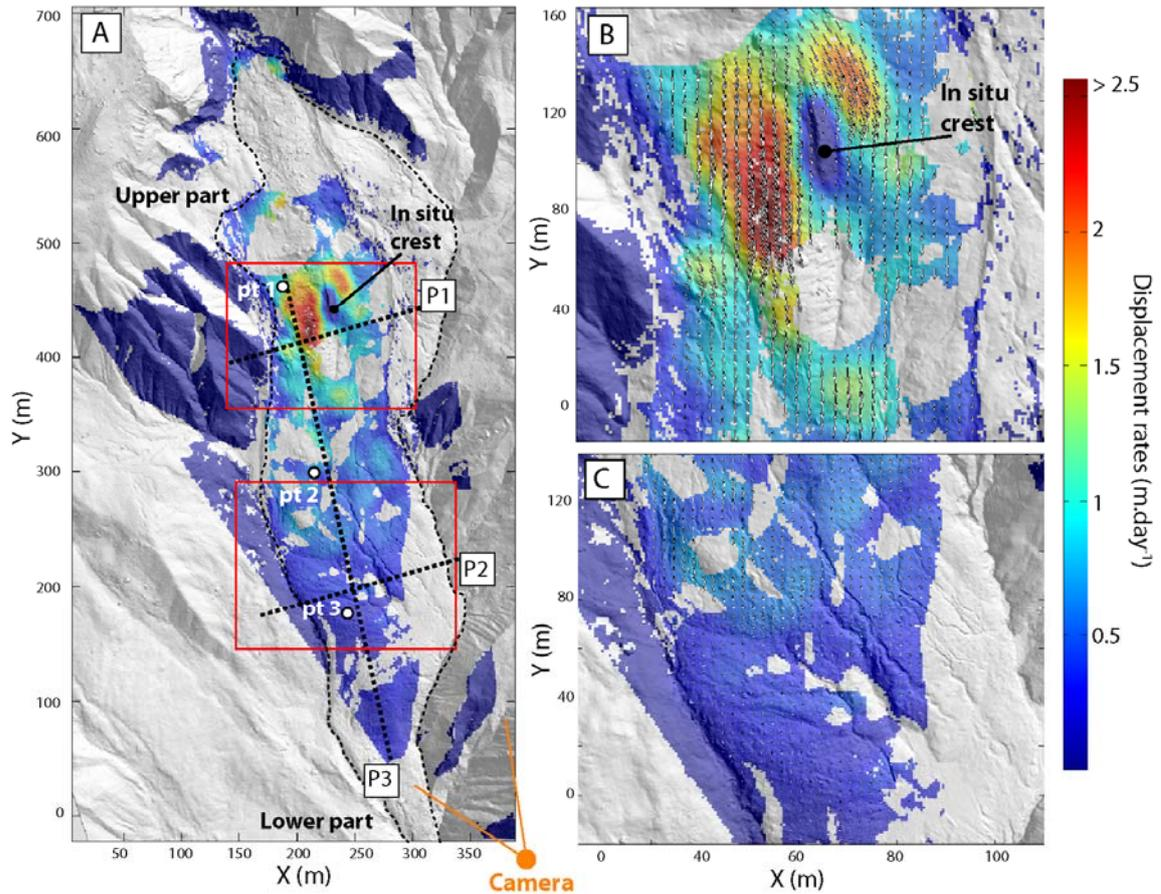
Fig. 9. Displacement rates map for the period 1<sup>st</sup> – 4<sup>th</sup> June 2008. (A) Displacement rates observed on the whole landslide. The profiles P1, P2 and P3 refer to Fig. 10 and the locations pt 1, pt 2 and pt 3 refer to Fig. 11. (B) Details on the displacement rates and displacement direction of the velocity amplitude and direction in the upper part. (C) Details on the displacement rates and displacement direction in the lower part.
