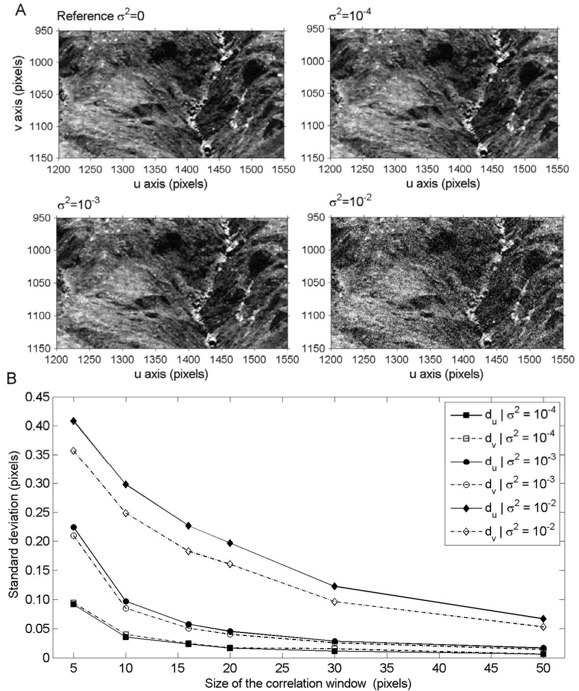
Fig. 12. Precision of the correlation algorithm. (A) Examples of different level of Gaussian noise created in the images of displacements (B) Precision of the hierarchical correlator in the  $u$  and  $v$  direction as a function of different levels of Gaussian noise ( $\sigma_n^2$ ) and different sizes of the correlation window.
