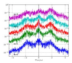
FIGURE 7. Partial energy frequency spectra  $\mathcal{E}_m(\varpi)$  of the magnetic field at the outer surface  $(1 < r < 1.024, 0.35 < \sin \theta < 0.6)$  for different m. a) Equatorially symmetric part. b) Equatorially-antisymmetric part. Frequencies are normalized by f, the rotation frequency of the inner sphere, and are shifted according to equation 3.3.  $Pm = 10^{-3}$ , Re = 2611 and  $\Lambda = 3.4 \times 10^{-2}$ .
