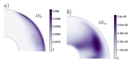
FIGURE 9. Time-and-azimuth-averaged meridional map of the energy of the fluctuations. a) Kinetic energy. b) Magnetic energy.  $Pm=10^{-3},~Re=2\,611$  and  $\Lambda=3.4\times10^{-2}$ . The energies are normalized by  $E_K^0=\frac{1}{2}\rho\left(2\pi f\right)^2b^2$ .
