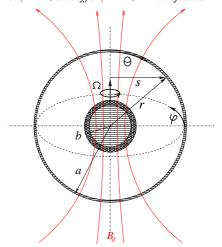
FIGURE 2. Sketch of the DTS experiment as modeled in this article. The inner sphere of radius b rotates around the vertical axis at angular velocity  $\Omega$ . It consists in a copper shell enclosing a permanent magnet, which produces the imposed dipolar magnetic field  $B_d$ . Liquid sodium of electric conductivity  $\sigma$  fills the gap between the inner sphere and the stainless steel outer shell of inner radius a. The spherical coordinate system we use is drawn.
