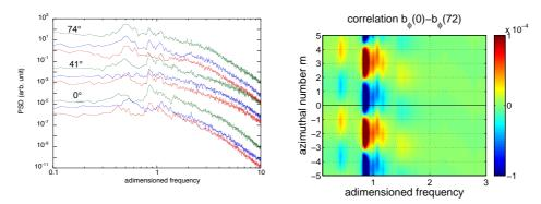
FIGURE 13. Same as figure 5 but for a simulation where the Lorentz force is nulled out for  $m \neq 0$ . Sharp spectral peaks are observed on all three components of the magnetic field. Neighbouring frequencies can have different azimuthal modenumber m.
