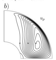
FIGURE 3. Time-averaged meridional slice of the velocity field. a) Angular velocity isovalues. Note the zone of super-rotation near the inner sphere. b) Meridional streamlines. The maximum meridional velocity is 0.4.  $Pm = 10^{-3}$ , Re = 2611,  $\Lambda = 3.4 \times 10^{-2}$ .
