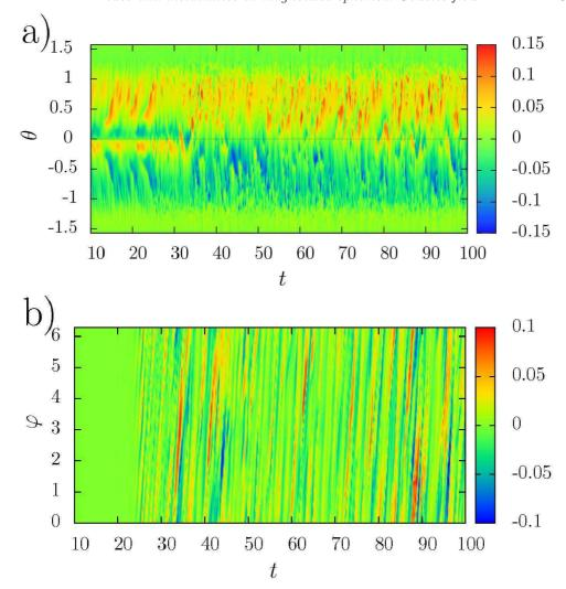
FIGURE 11. Spatio-temporal representation of the velocity fluctuations in the simulation at radius r=0.95.  $Pm=10^{-3}$ ,  $Re=2\,611$  and  $\Lambda=3.4\times10^{-2}$ . a)  $V_{\theta}$  isovalues of the axisymmetric flow (m=0) in a latitude-time plot. b)  $V_{\varphi}$  isovalues at 10° latitude in an azimuth-time plot (m=0 term removed). Velocities are normalized by the reference velocity  $\Omega b$ . Time is given in rotation periods.
