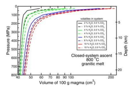
Fig. 16. Magma volume as a function of pressure at 800 °C. At high pressures, the fluid phase is minor and the volume of all the modeled rhyoltic volumes are similar. However, as pressure decreases and fluid exsolves from the melts, the volume becomes significant, particularly at pressures below approximately 200 MPa. This large volume increase may be responsible for the cracking of country rocks, loss of the volatile phase from the melt, and the formation of ore deposits (e.g., Burnham, 1979b).
