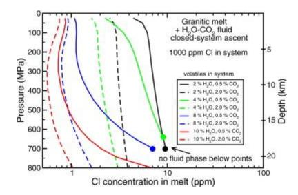
Fig. 14. Chlorine concentration in the rhyoltic melt during ascent based upon the measurements of Shinohara et al. (1989). The fluid phase scavenges almost all of the chlorine from the melt and probably ore metals bound to chlorine. The effects of pressure on the partition coefficient seen in Fig. 10 do not have a significant effect of the behavior of chlorine because at all conditions the modeled partition coefficient remains above 100.
