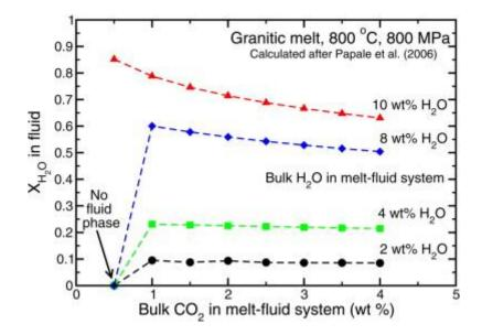
Fig. 11. Concentrations of water and carbon dioxide in fluids coexisting with a rhyolitic melt at 800 MPa, 800 °C calculated using the model of Papale et al. (2006). For  $CO_2$  concentrations of 0.5 wt.% in the system composed of fluid + silicate melt no fluid phase exists, except when the water concentration is above approximately 9.5 wt%. Please see the text for further discussion of this model.
