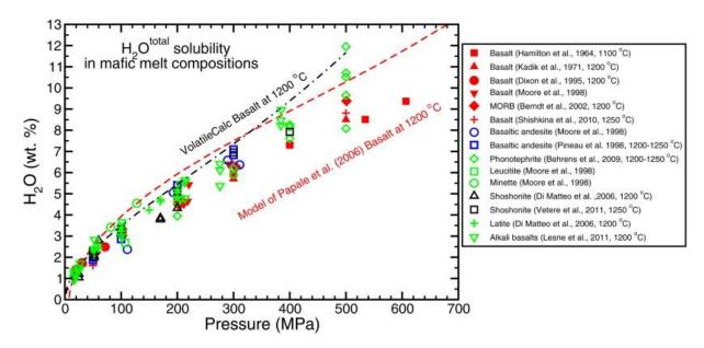
Fig. 6. Water solubility in natural mafic composition melts. Measured solubilities (data points) and the the solubility modeled for the basaltic melt of Hamilton et al. (1964) at 1200 °C using the model of Papale et al. (2006) and the water solubility for a basaltic melt with 49 wt.%  $SiO_2$  calculated with volatilecalc (Newman and Lowenstern, 2002) are plotted. Uncertainties in the measurements are similar to the size of the symbols.
