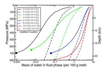
Fig. 15. Mass of the fluid phase exsolved from a silicic melt during ascent. The mass of the fluid phase increases significantly for magmas with low concentrations of volatiles during ascent, but the increase is less spectacular for magmas rich in volatiles because many volatiles exsolve at higher pressure. Nevertheless, magmas with larger concentrations of volatiles exsolve larger masses of fluids as required by the conservation of mass.
