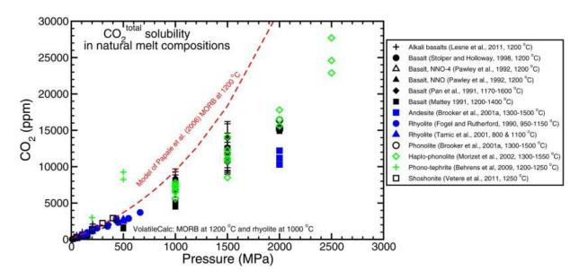
Fig. 7. Carbon dioxide solubility in natural melt compositions. Measurement uncertainties are shown for the data of Pan et al. (1991). Carbon dioxide solubilities calculated by volatilecalc and by the Papale et al. model for a mid-ocean ridge basalt (MORB) at 1200 °C are also plotted.
