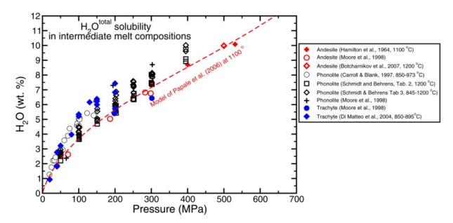
Fig. 5. Water solubility in natural intermediate composition melts. Both measured solubilities (data points) and the solubility modeled for the andesitic melt of Hamilton et al. (1964) at 1100 °C using the model of Papale et al. (2006) are plotted. Uncertainties in the measurements are similar to the size of the symbols.
