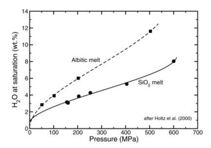
Fig. 2. Comparison of the solubility of water in an albitic melt and in a melt of pure  $SiO_2$ . The lower water solubility in silica melt is hypothesized to be due to the lack of exchangeable cations (e.g.,  $Na^+$ ) in the theory of Burnham. Measurement uncertainties are approximately the size of the symbols. Please see text for a further discussion. Data are from Holtz et al. (2000).
