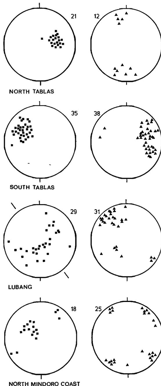
Fig. 5. Stereographic diagrams of Lubang, North Mindoro coast, and north and south Tablas areas. The squares represent pole projections of foliation planes. The triangles represent the projection of stretching lineations. The N150°E trending line on the foliation pole diagram of Lubang is the axis of the upright fold. Numbers of measurements given next to each lower hemisphere projection.
