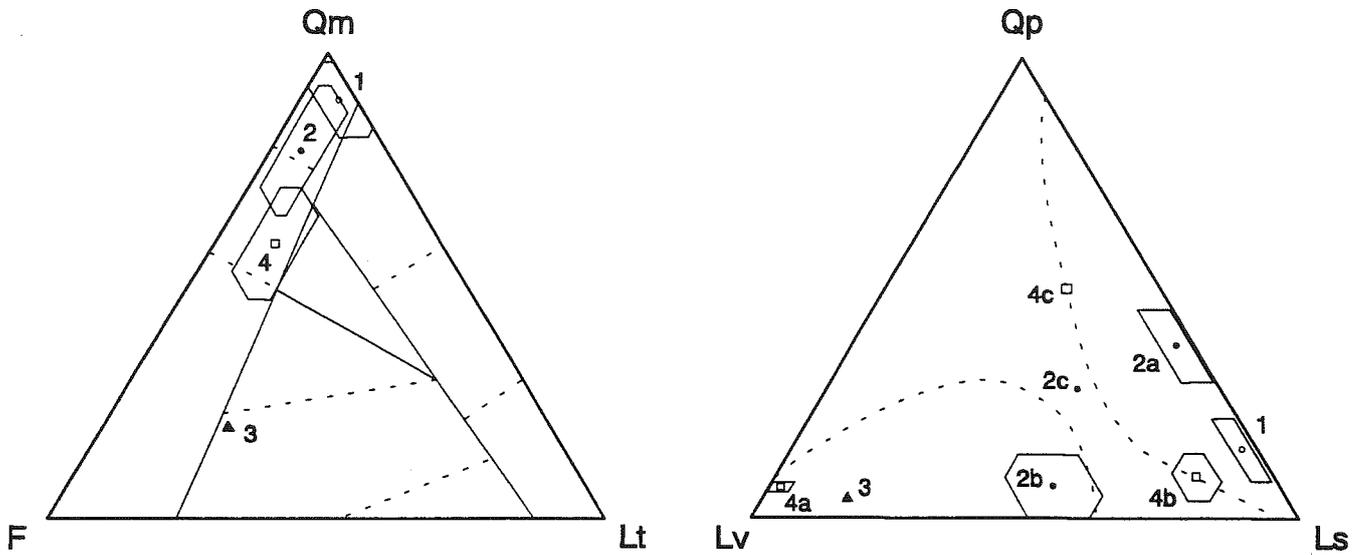
Figure: Distribution of mean detrital modes (plus one standard deviation) of sandstone suites derived from Upper Devonian and Carboniferous units in the Altiplano of Bolivia. Data in QpLvLs diagram is only for samples with  $Lt \geq 9$ . 1, Upper Devonian; 2, Kasa Fm.; 3, Siripaca Fm.; 4, Yaurichambi Fm.
