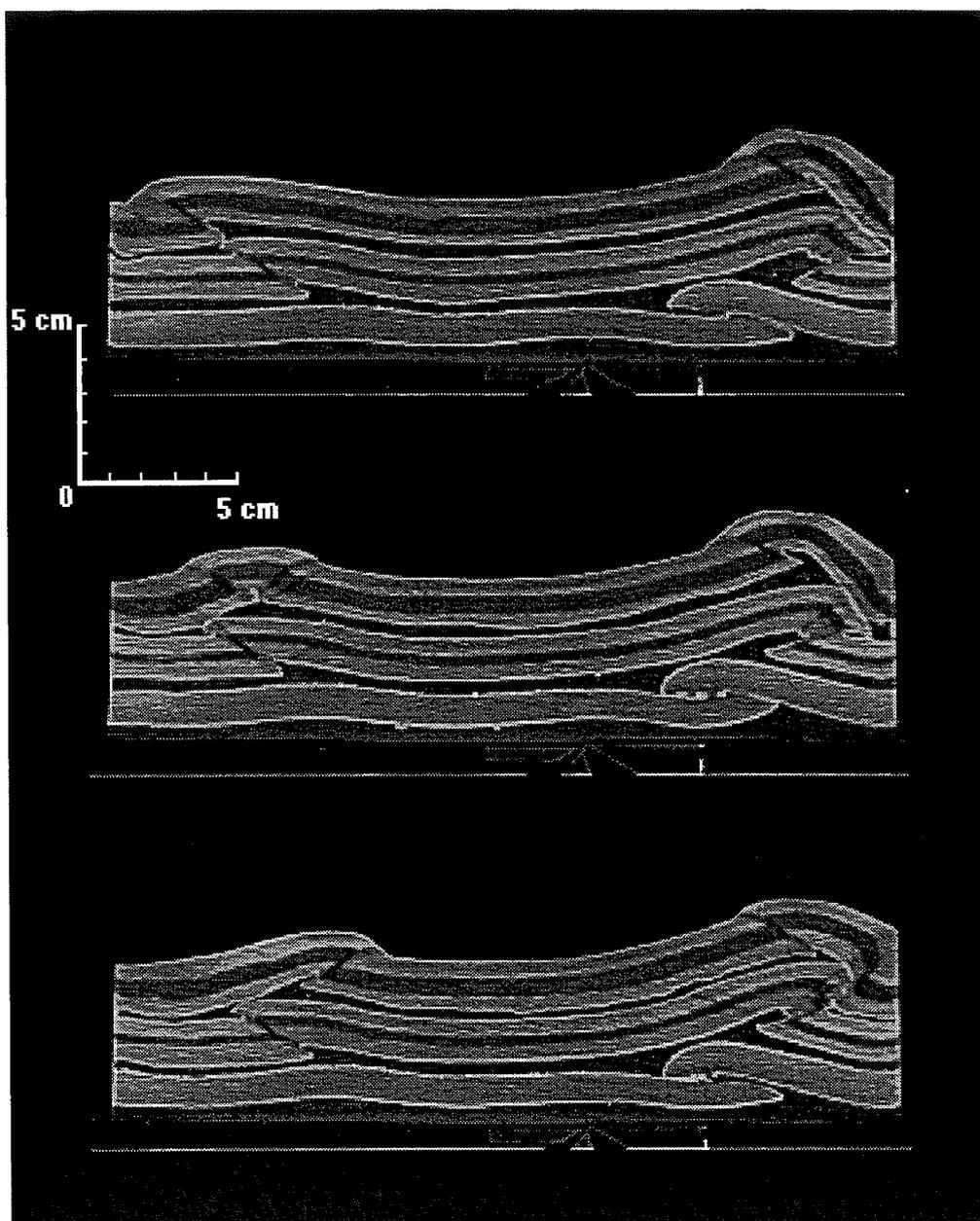
Fig. 1 : Serial cross-sections (computerised x-ray tomography images) of a "three ductile interbedded layers" model showing "fish tail" structures and lateral changes of thrust vergence.
