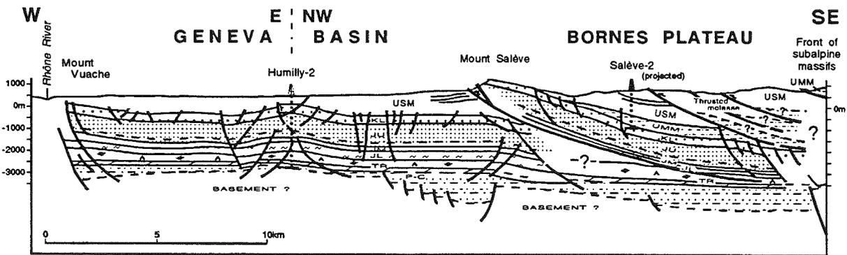
Fig. 3 : Geological cross-section derived from seismic data
