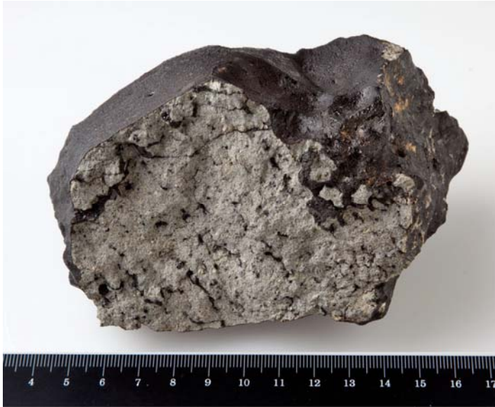
Fig. 1. The Natural History Museum (London) stone. This 1.1 kg stone (BM.2012,M1) exhibits a black fusion crust with glossy olivines. The olivine macrocrysts (pale green) and the numerous black glass pockets and veins, are characteristics of this shergottite. The scale is in cm.
