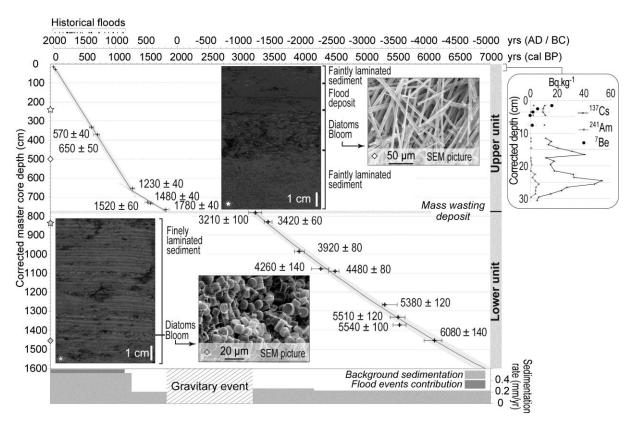
Figure 4: Age-depth model, correlation with historical floods, sedimentation rates and sedimentological units. Stars and diamonds locate the depths of the pictures presented. <sup>137</sup>Cs, <sup>241</sup>Am and <sup>7</sup>Be of the top of the core are provided on the right.
