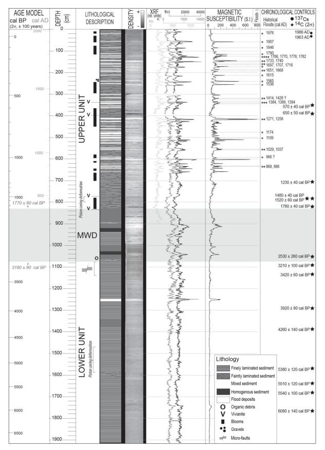
Figure 3: Core description, lithology and physical parameters (density, MS, and XRF – Rb, Ti, K), stratigraphic location of the <sup>137</sup>Cs and <sup>14</sup>C ages and of the historical floods. Mass
