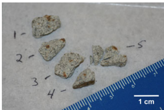
Fig. 1. Photograph of the Antarctic L5 ordinary chondrite GRO 95540 broken up into five pieces using a Parafilm sealed hand hammer.
