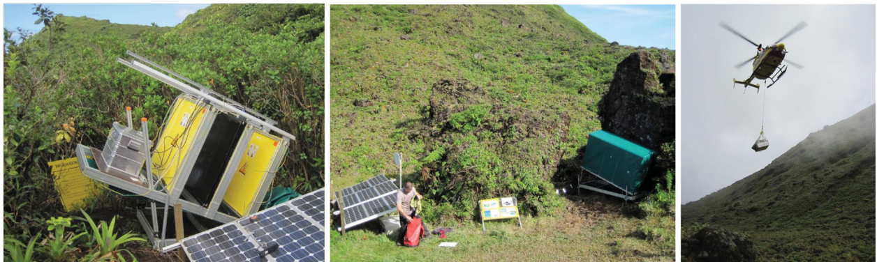
Figure 3. Left-hand side: view of the telescope equipped with three scintillator matrices. The iron shielding is the black plate placed against the central matrix. The aluminium box contains electronic devices: data logger, DC–DC converters, reference clock, ethernet switch, main computer. Middle: general view of the installation at the Roche Fendue site. Three solar units each with peak power of 270 W are necessary because of the quasi permanent cloudy weather. The telescope is equipped with its green tarpaulin and ready for measurements. Right-hand side: moving of the telescope from the Ravine Sud site toward the Roche Fendue place.
