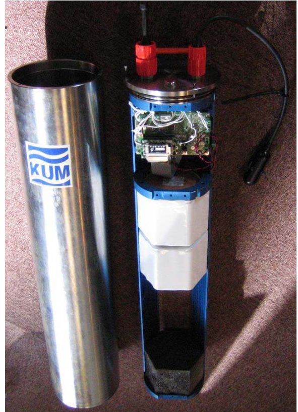
Figure 5 Titanium cylinder housing the batteries, electronic board and data storage (hard disk drive)
