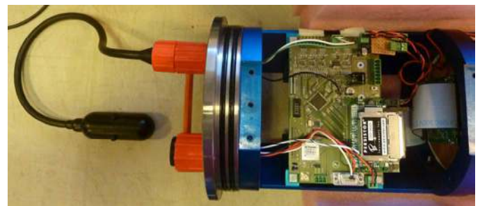
Figure 6 Hydrophone electronic board and sensor.
