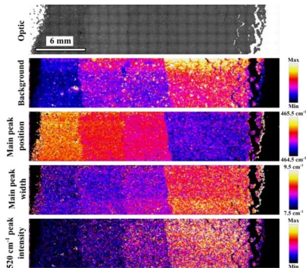
Figure 3. Raman analyses of quartz powders. (a) Photography and large area Raman maps (decreasing in grain size from left to right) showing background level, position of the main peak, width of the main peak and intensity of the peak at 520 cm<sup>-1</sup>.
