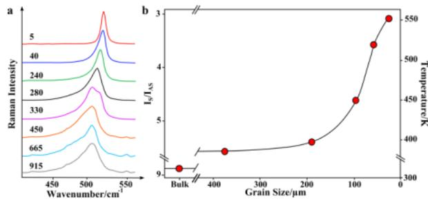
Figure 8. (a) Main peak of silicon corresponding to different laser powers (in kW/cm<sup>2</sup>) acquired using the WITec system on the <40 μm grain size powder. (b) Stokes and Anti-Stokes intensity ratio and associated local temperature with respect to the grain size distribution of the silicon sample measured using the iHR320 system interfaced with the RLS simulator.
