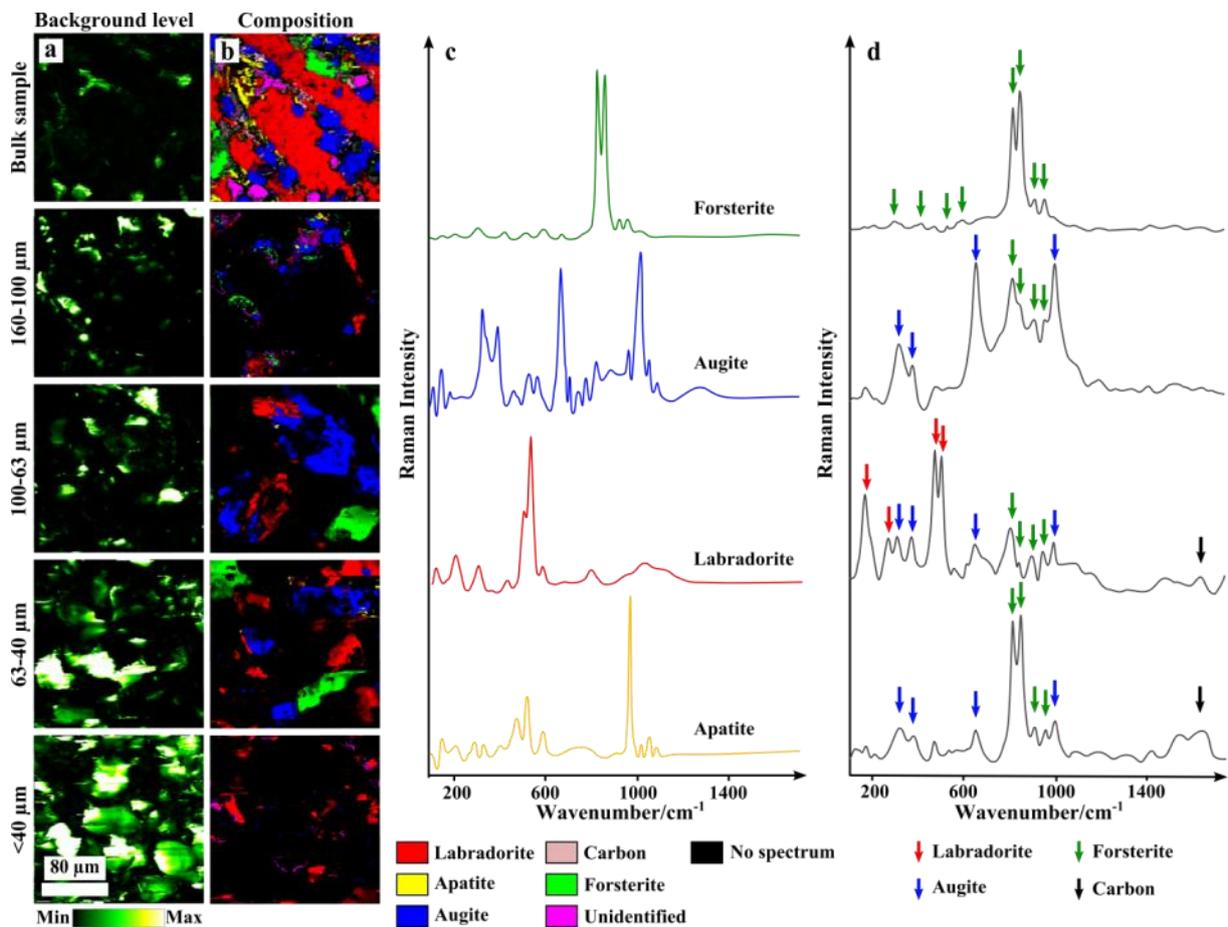
Figure 5. Background level (a) and compositional Raman maps (b) of bulk and powdered basalt samples (scan size 200x200  $\mu\text{m}^2$ ) acquired using the WITec system. Single Raman spectra of 160 to 100  $\mu\text{m}$  grain sized basalt powder (c) collected using the line scan method
