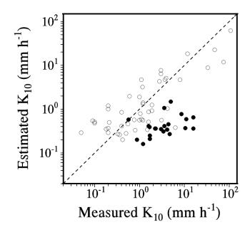
**Fig. 2.** Measured and predicted saturated matrix hydraulic conductivity. Data are taken from Jarvis et al. (2002). Predicted values are calculated using Eq. (2), and  $\theta_{10}$  and *n* are predicted by HYPRES. Solid symbols represent data obtained by three of the ten researchers.
