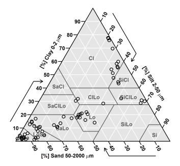
Fig. 1. Textures of the different horizons of the 16 soils used for our study, represented over USDA Soil Texture Triangle classes: "Cl" means "Clay" or "Clayey"; "Si" means "Silt" or "Silty"; 'Sa" means "Sand" or "Sandy"; and "Lo" means "Loam" or "Loamy".
