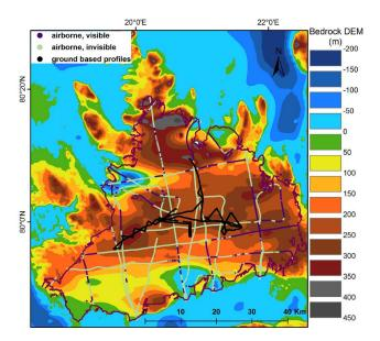
**Fig. 3.** Digital elevation model for the bedrock elevation, overlaid are the ground-based (black) and airborne radar profiles (blue, gray: lack of bed return). In the land areas, this map is completed with the NPI map and in sea areas with the IBCAO data. However, these data were not used to establish the bedrock map from the individual profiles.
