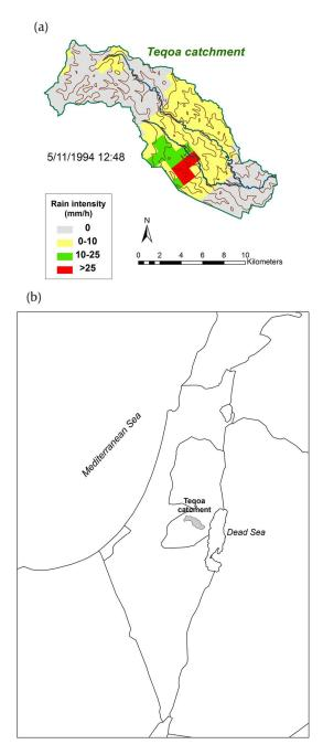
**Fig. 6.** Teqoa Event occurring in November 1994. (a) Radar-based rainfall intensities over the Teqoa catchment for 12:48 (local time), brown contour lines represent elevation (0–900 m in 100 m intervals), and, (b) general location of the Teqoa catchment.
