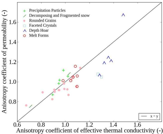
**Fig. 3.** Anisotropy coefficient computed for the intrinsic permeability  $A(\mathbf{K})$  vs. that for the effective thermal conductivity  $A(\mathbf{k}_{\text{eff}})$  for the 35 samples considered in this study. Symbols and colors correspond to the ICSSG (Fierz et al., 2009).
