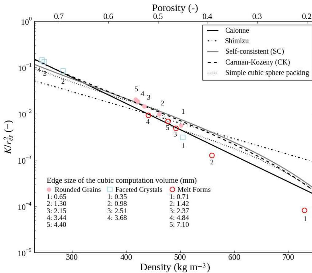
**Fig. 6.** Dimensionless permeability versus snow density for three snow samples. Symbols and colors correspond to the ICSSG (Fierz et al., 2009). For a given sample, each symbol represents a particular volume from which  $K$ , SSA and  $\rho_s$  were computed. The largest volume corresponds to the total volume of the sample. Analytical models and fits are also plotted.
