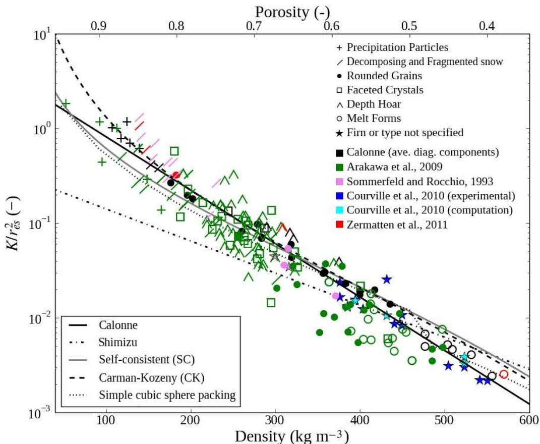
**Fig. 4.** Dimensionless permeability vs. snow density. Our  $K^*$  values (in black) are compared to results from other studies (in color). Symbols correspond to the ICSSG (Fierz et al., 2009), excepting stars which are used when firm is considered or when the snow type is not specified in the paper. Analytical models and fits are also plotted.
