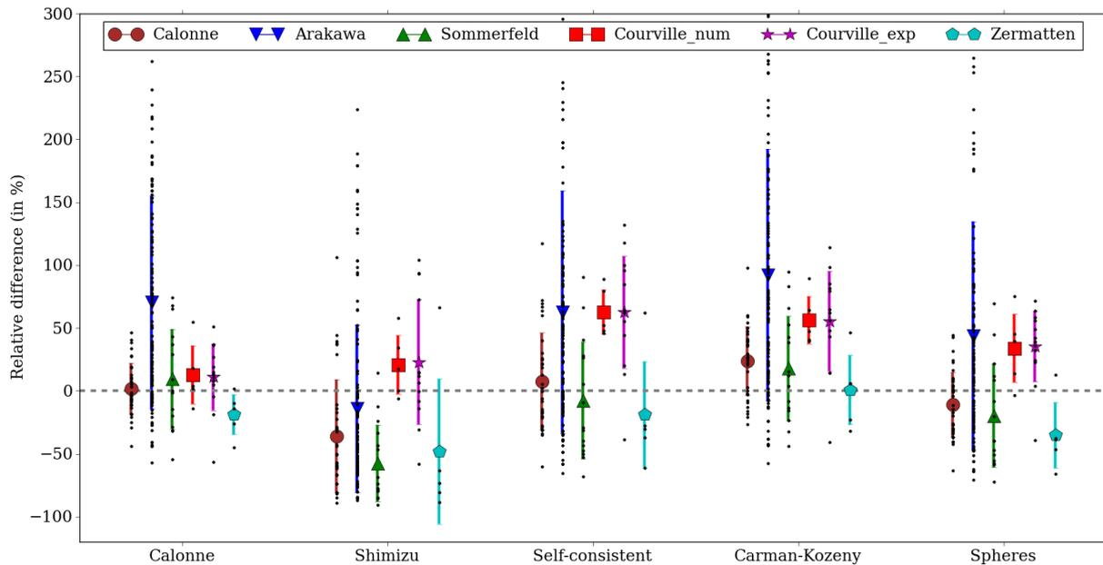
**Fig. 5.** Overview of the relative differences between experimental or numerically computed values of the intrinsic permeability of snow from six datasets (colors) and their estimates based on the corresponding snow density and equivalent sphere radius using various regression or analytical curves (x-axis). Black dots refer to individual measurements of relative residual. The mean and standard deviation of the relative differences are indicated as symbols and error bars, respectively.
