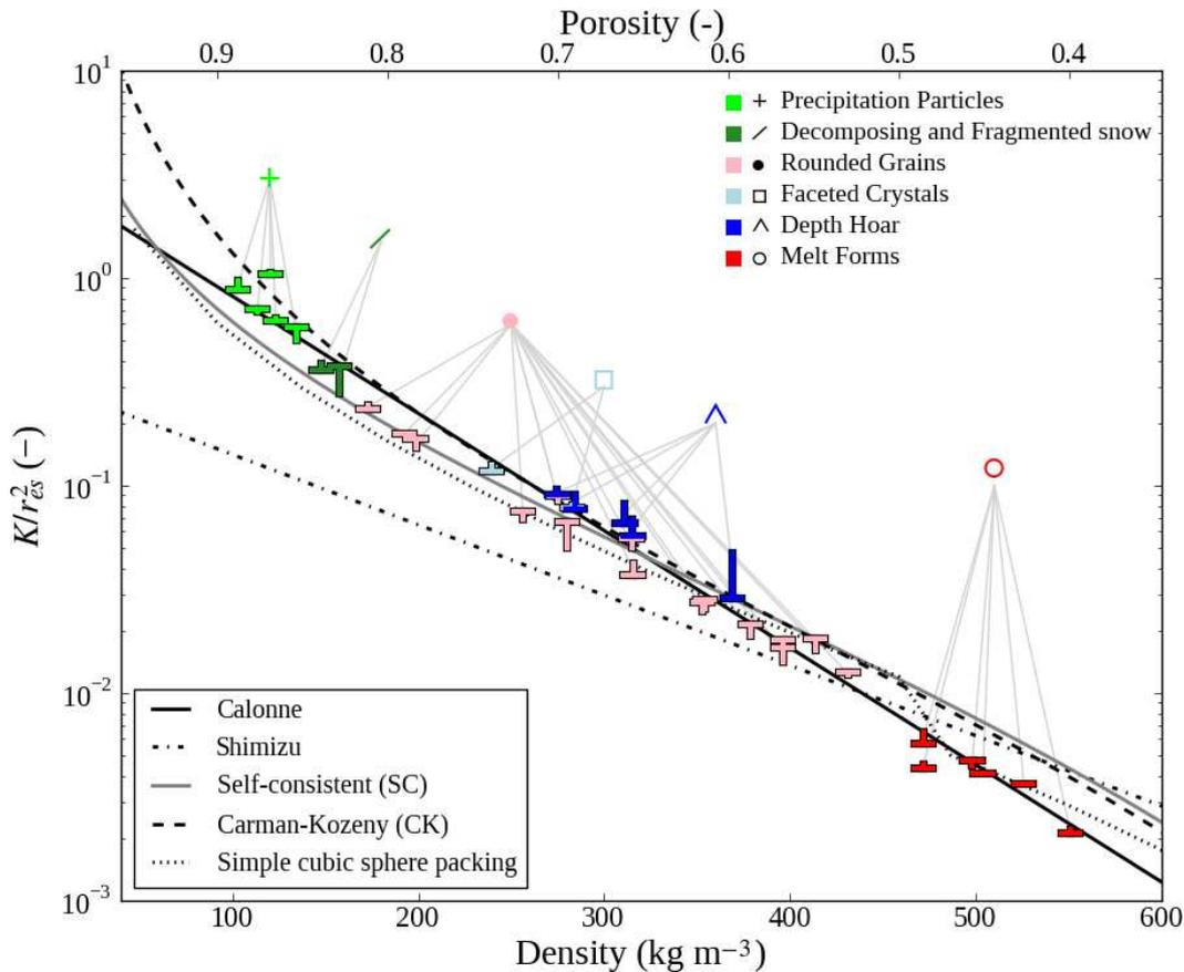
**Fig. 1.** Dimensionless permeability vs. snow density. “T” symbols indicate the values obtained by our numerical computations. Tips and horizontal bars of the “T” shapes represent the vertical ( $K_z^*$ ) and horizontal ( $K_{xy}^*$ ) components of  $\mathbf{K}^*$ , respectively. Colors correspond to the ICSSG (Fierz et al., 2009). Analytical models, numerical computations and fits are also plotted.
