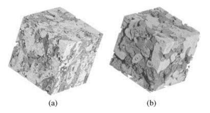
Fig. 2.: Area of interest of 256<sup>3</sup> voxels selected from two different stone samples: RFF sample (a) and RF sample (b).
