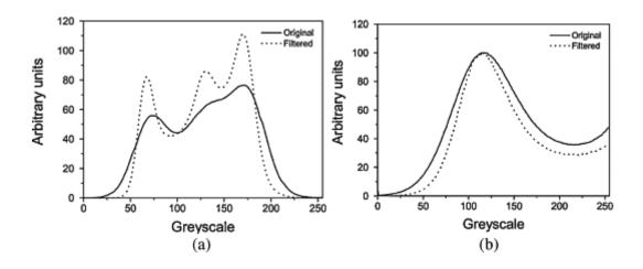
Fig. 5.: Grayscale histograms recorded for a stone sample (a) and a bone sample (b), compared to the histogram of the filtered samples.
