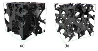
Fig. 3.: Area of interest of of 256<sup>3</sup> voxels selected from two different bone samples: OA sample (a) and OP sample (b). Bone material is in gray color while pore material is in white.
