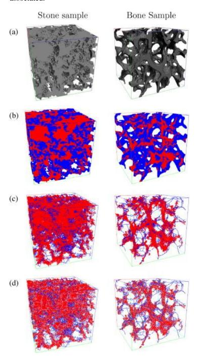
Fig. 6. : 3D porous media: one-connected objects (a), classified volumes, (b) hybrid skeletons, (c) and the final individualized skeletons (d). Rod voxels are in blue, plate voxels are in red while node and border voxels are in green.
