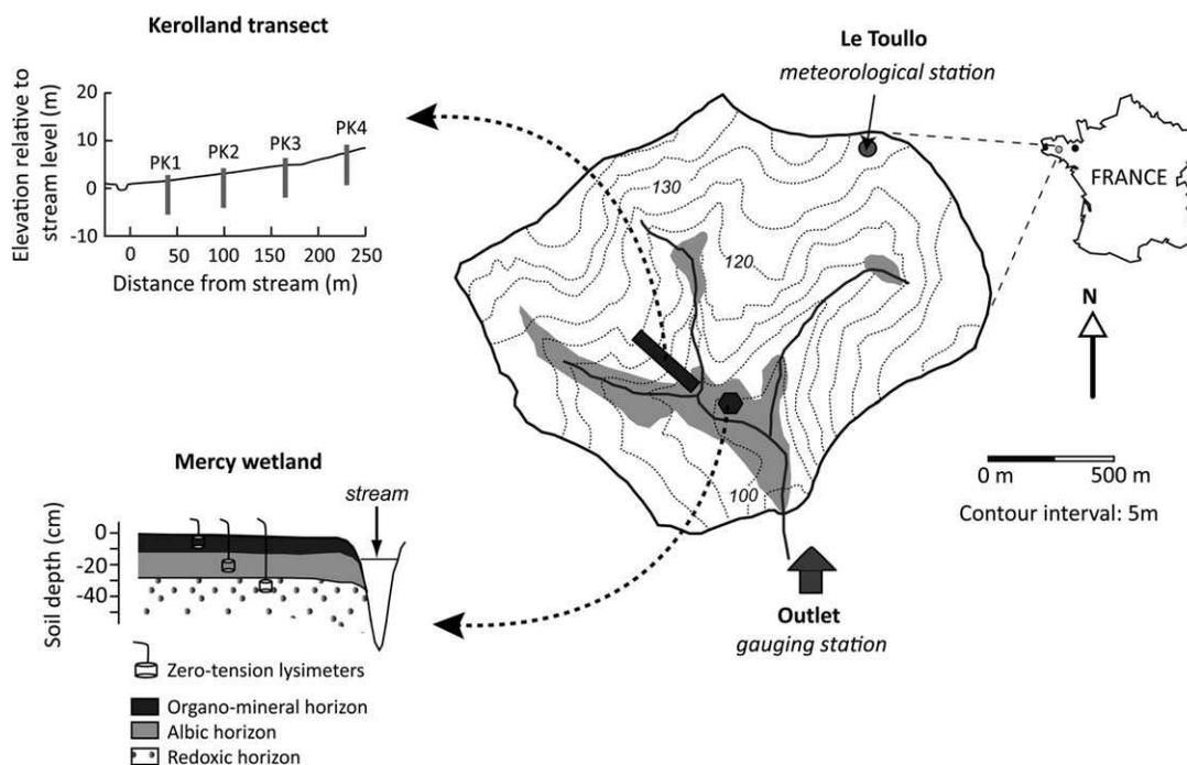
**Figure 1.** Location map of the Kervidy-Naizin experimental catchment (Brittany, France) showing the different instrumented sites. Gray areas located along the stream channel network indicate the maximum extent of wetland zones.
