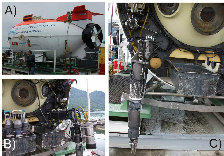
Fig. 2. A) One of the MIR submersibles on the barge in Lake Geneva. B) MIR 1 prepared for the survey on 12 Aug 2011. One of the baskets was loaded with sediment coring tubes (left) and the other one carried Nimrod . Fixed pieces of wood secured Nimrod in the shown position to enable easy access by the robotic claw. During transit, the baskets were shifted further under the main body of the MIR. The video camera is attached to the portside robotic arm. C) Starboard robotic arm of MIR 1, which was used for deployment and recovery of Nimrod .
