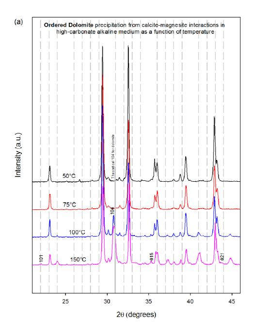
Figure 1. Experimental XRD patterns for dolomite precipitation via simultaneous dissolution of calcite and magnesite. 101, 015 and 021 are typical superstructure reflections for dolomite in the 20-45 2th range (ICDD 036-0426). Influence of temperature and nature of interacting fluid. (a) reaction in high-carbonate alkaline solution and (b) in high-purity water.
