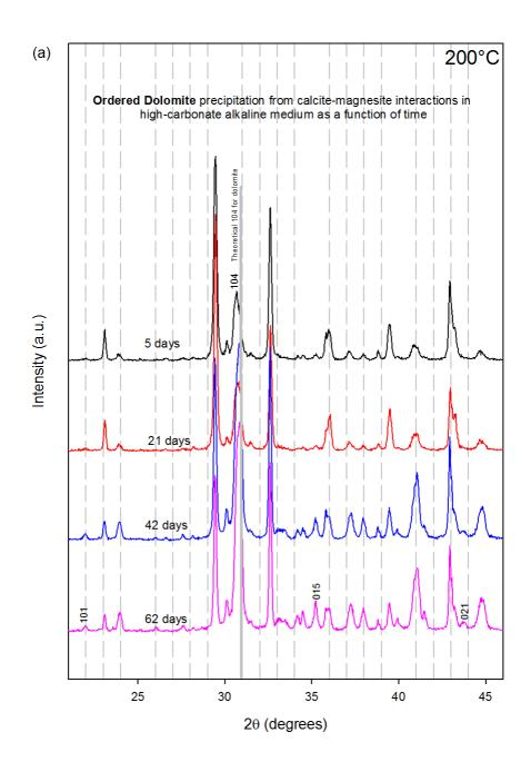
Figure 4. Experimental XRD patterns for dolomite precipitation via simultaneous dissolution of calcite and magnesite. 101, 015 and 021 are typical superstructure reflections for dolomite in the 20-45 2th range (ICDD 036-0426). Kinetic behavior at (a) 200°C and (b) 150°C.
