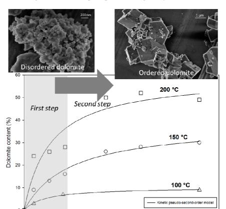
**Synopsis:** This study provides new experimental conditions to which dolomite can be formed in hydrothermal systems via simultaneous dissolution of calcite and magnesite. Herein, the dolomite formation was co-promoted by temperature and high-carbonate alkalinity. The activation energy for this reaction pathway ( ) is 29 kJ/mol.
