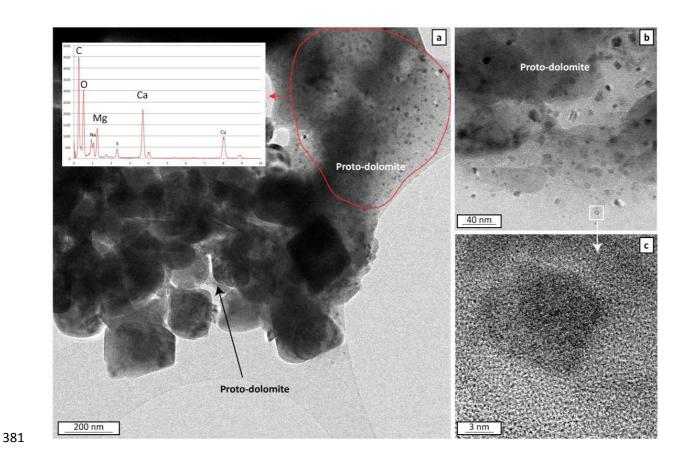
Figure 3. Bright field image of a) proto-dolomite mixed with calcite and magnesite grains (from run 16) (inset: EDS spectrum extracted from STEM chemical mapping), magnification of proto-dolomite where nanoparticles are scattered in an amorphous gel, c) high-resolution of a crystalline nano-particle.
