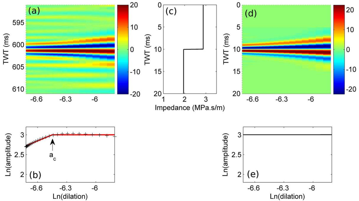
**Figure 3.** (a) and (b) Source-corrected WR and ridge function of BS2, respectively. The ridge function (stars) is approximated by two segments (red lines). (c) Synthetic impedance profile of a homogeneous half-space medium (Heaviside-like discontinuity). (d) and (e) Theoretical WR and ridge function, respectively.
