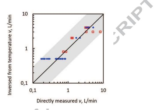
Figure 8: Comparison between flowmeter measurements and velocity values inverted from temperature measurements. Blue markers correspond to ambient flow conditions, while red markers correspond to cross-borehole pumping conditions. Note, that this plot also demonstrates the variability of the flow measurements inside borehole sections due to the tool error and/or variations in borehole diameter.
