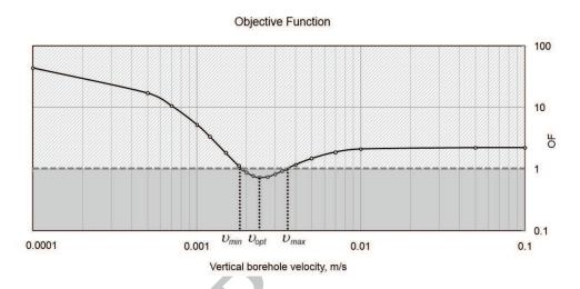
Figure 7: Example of the objective function versus the vertical borehole flow velocity. The minima of the objective function corresponds to the optimal flow velocity  $(v_{opt})$ , and all the solutions in the range  $(v_{min}, v_{max})$  are acceptable.
