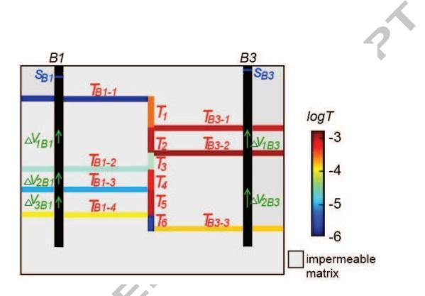
Figure 10: Inferred fracture transmissivities (T) and connectivities between and around B3-B1 borehole pair. Observation well drawdowns during cross-borehole pumping s are shown by blue lines. Variations of vertical velocities during cross-borehole pumping  $\Delta v$  in observation boreholes are shown by green arrows.
