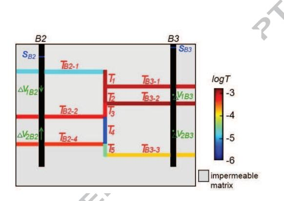
Figure 11: Inferred fracture transmissivities (T) and connectivities between and around B2-B3 borehole pair. Observation well drawdowns during cross-borehole pumping s are shown by blue lines. Variations of vertical velocities during cross-borehole pumping  $\Delta v$  in observation boreholes are shown by green arrows.
