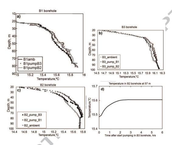
Figure 5: Temperature tomography experiment. Steady-state temperature profiles measured in B1 well when pumping in B2 and B3 wells (a). Steady-state temperature profiles measured in B2 well when pumping in B1 and B3 wells (b). Steady-state temperature profiles measured in B3 well when pumping in B1 and B2 wells (c). Example of temporal evolution of temperature in B2 at 57 m depth (d).
