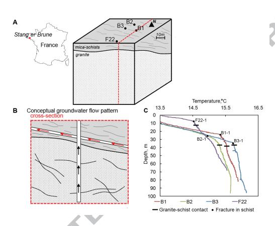
Figure 4: A. Location of the Stang-er-Brune study site, boreholes array configuration and geology of the site. B. Conceptual hydrothermal setting: temperature profile affected by groundwater flow of warmer origin, by localized flow of warmer or cooler origin in narrow fractures and by vertical flow in the borehole itself. C. Temperature profiles measured at the site under the ambient flow conditions.
