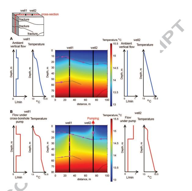
Figure 1: Illustration of a typical groundwater flow and temperature fields for a pair of boreholes connected by one main flow path and intersected by one disconnected fracture each borehole under ambient (A) and pumping (B) flow conditions. The velocity field and temperature field are computed using 2D model.
