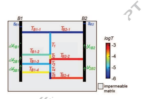
Figure 9: Inferred fracture transmissivities (T) and connectivities between and around B1-B2 borehole pair. Observation well drawdowns during cross-borehole pumping s are shown by blue lines. Variations of vertical velocities during cross-borehole pumping  $\Delta v$  in observation boreholes are shown by green arrows.
